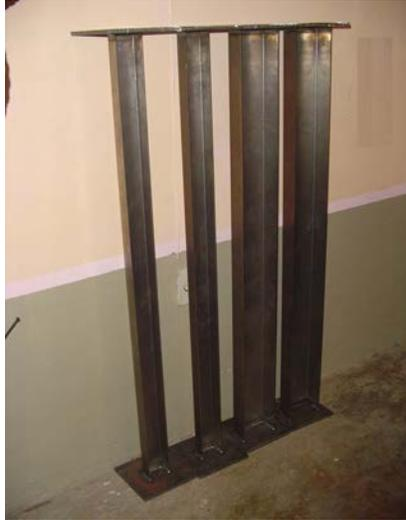
Fig. 8–View of four channel column used in experimental tests (U110x55x1.2 and U65x35x1.5)
