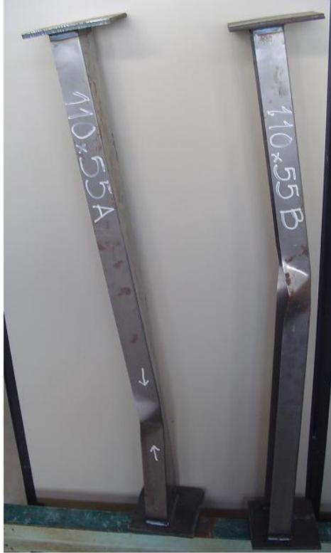
Fig. 10–Section already tested showing deformation for local buckling
