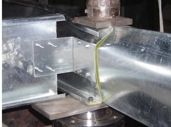
Figure 17: Web Crippling at the Specimen Failure
