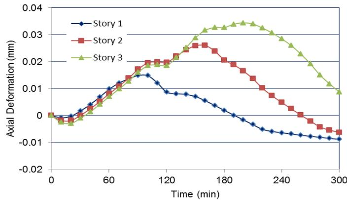
Figure 12: Axial deformation of the CFHSS columns as a function of fire exposure time corresponding to Case 11 analysis
