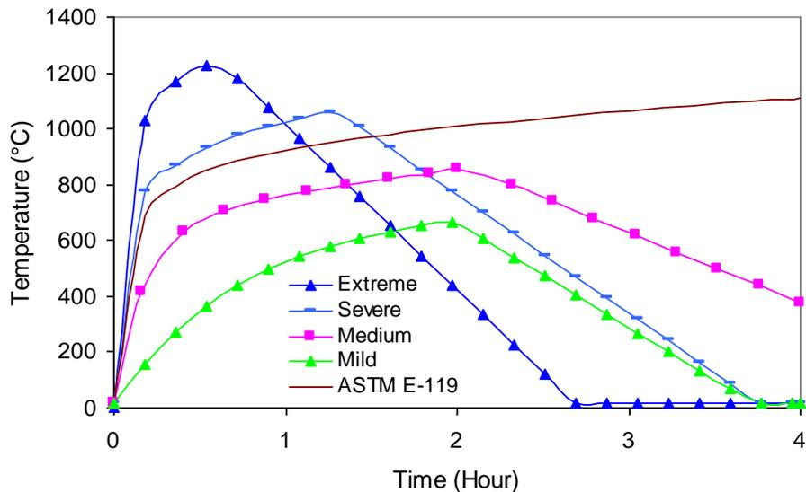
Figure 6: Possible fire scenarios used in the fire resistance analysis
