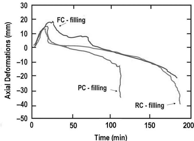
Figure 1: Axial deformation in CFHSS columns as a function of time
