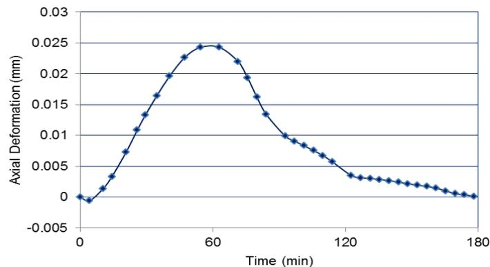
Figure 10: Axial deformation of the CFHSS column as a function of fire exposure time corresponding to Case 8 analysis
