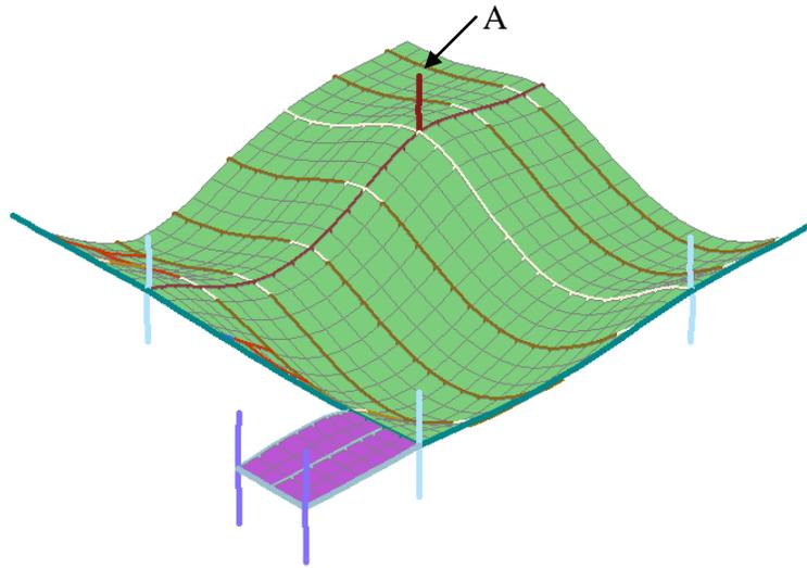
Figure 7: Deflected shape under service loads and ambient temperature (scale 1:125)
