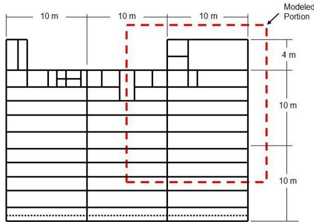
Figure 3: Framing plan for the steel framed building used to illustrate application of the developed methodologies
