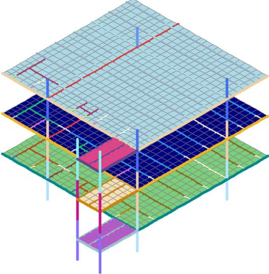
Figure 5: Three story numerical model of selected building
