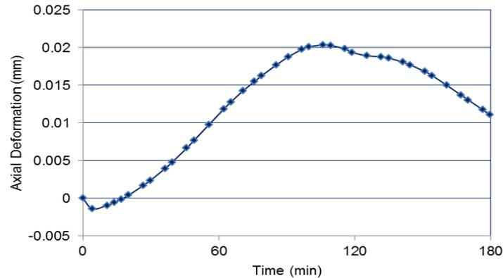
Figure 11: Axial deformation of the CFHSS column as a function of fire exposure time corresponding to Case 9 analysis
