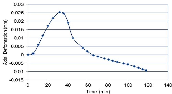
Figure 9: Axial deformation of the CFHSS column as a function of fire exposure time corresponding to Case 3 analysis
