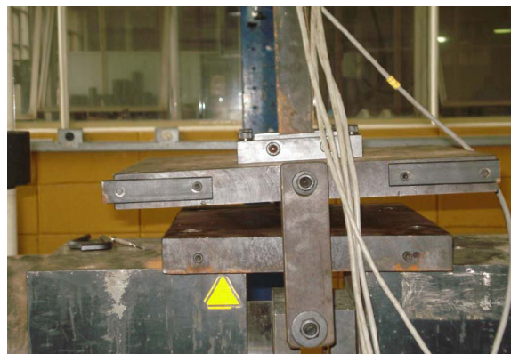
Figure 2: Typical end support arrangement in a pin-ended column test – “rigid link” and “cylindrical hinge”
