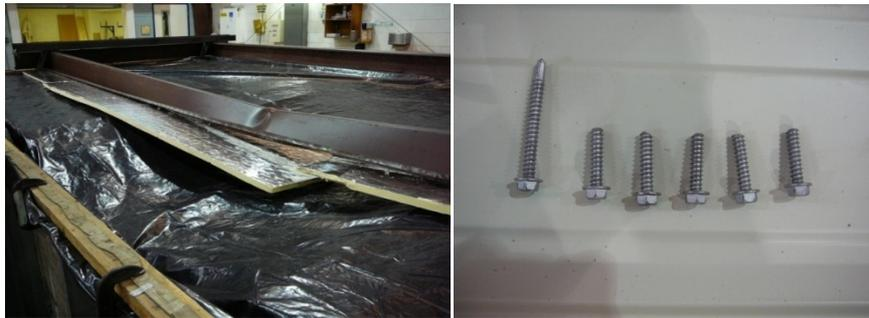
Figure 10: Failure mode in the test with 25.4 mm of rigid board
