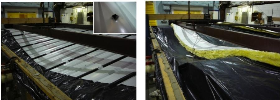
Figure 9: Panel pull-over failure in the bare panel tests
