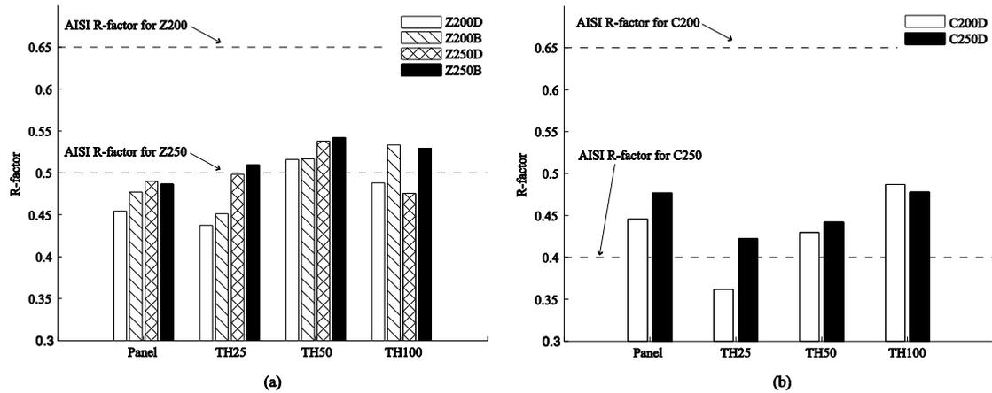
Figure 19: Influence of rigid board thickness on R-factors for (a) Z-sections and (b) C-sections
