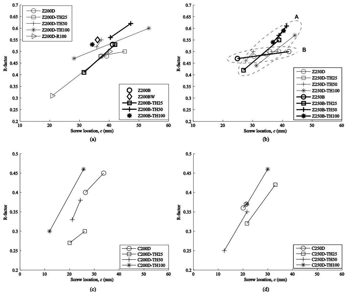
Figure 15: R-factor as a function screw location (a) Z200 (b) Z250 (c) C200 (d) C250
