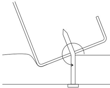
Figure 11: Screw bending due to existing of rigid board
