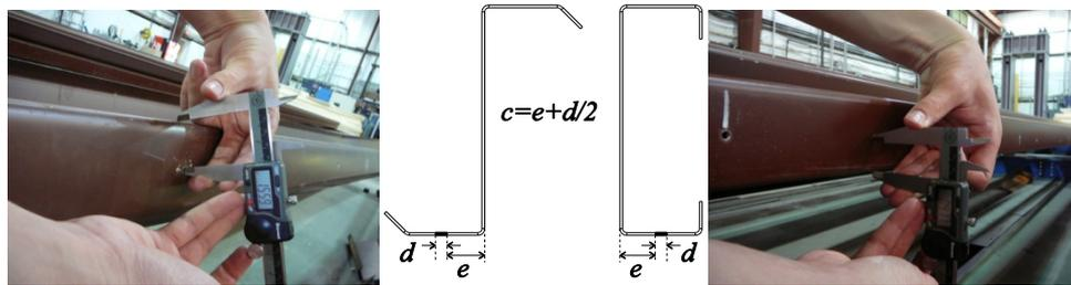
Figure 7: Screw location  $c$  measurement
