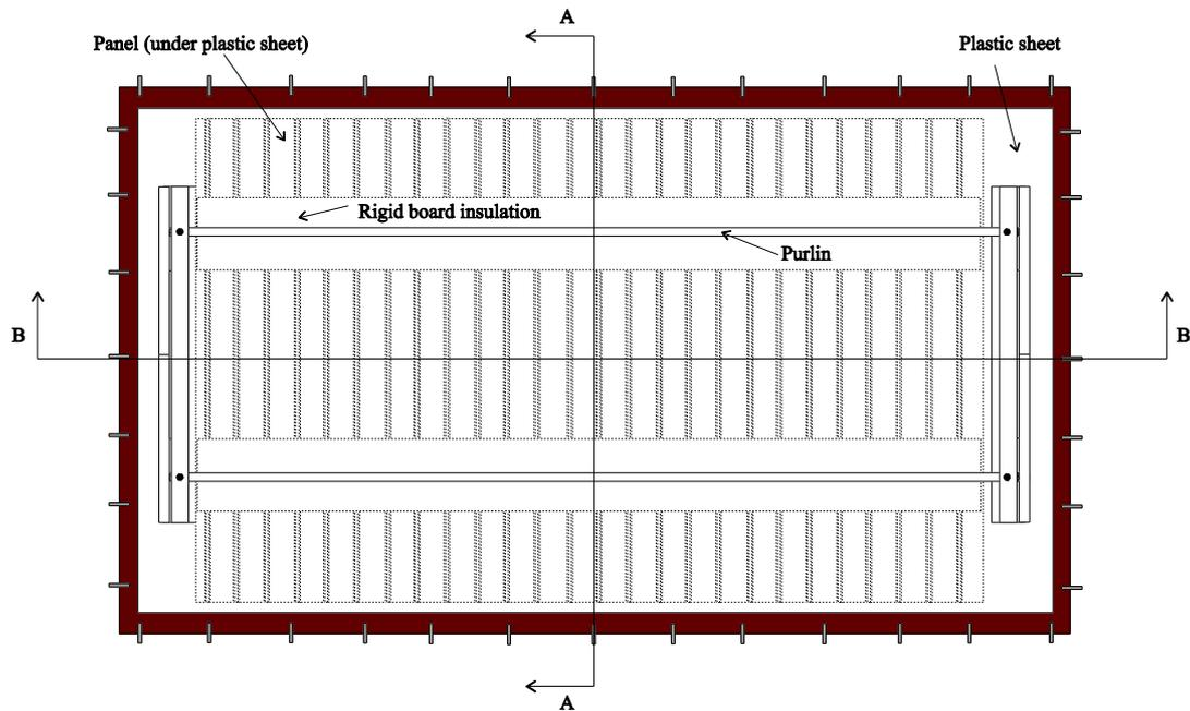
Figure 3: Test setup plan
