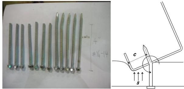
Figure 14: When  $c$  is small, the resisting moment is small and the screws break
