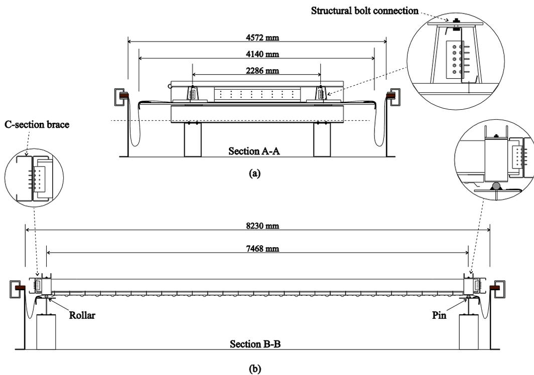
Figure 4: Test setup (a) section A-A (b) section B-B in Fig. 3
