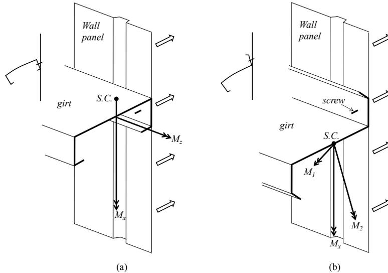
Figure 1: Girts rotation due to (a) torsion in a C-section from the load eccentricity, and (b) biaxial bending in a Z-section
