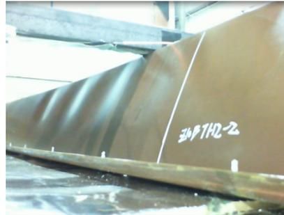
Figure 13: Local buckling during the test of slender cross section
