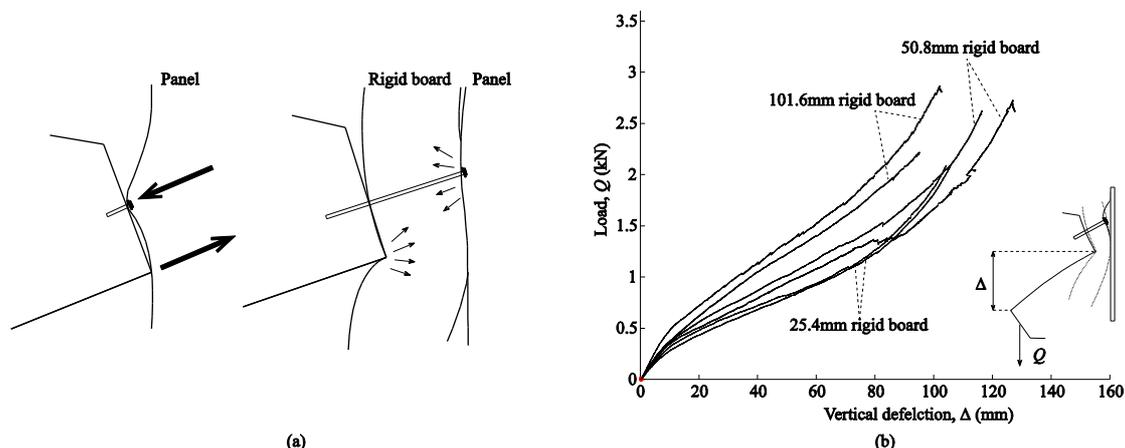
Figure 2: Rigid board influences girt rotational restraint: (a) fastener force spreads out across panel, and (b) girt rotational restraint is trilinear (Gao and Moen 2012b)
