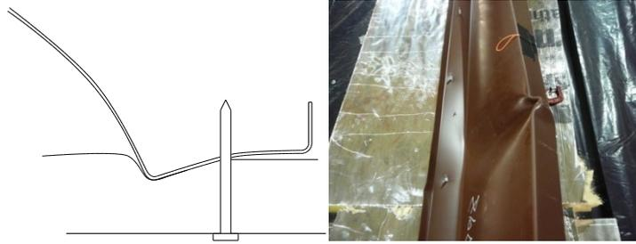
Figure 12: Deformation of slender cross section during the test
