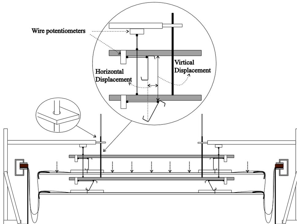
Figure 6: Instrumentation
