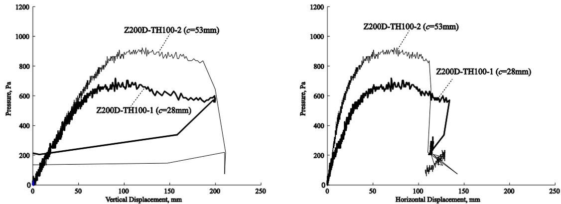
Figure 8: Effect of screw location  $c$  on the girt load-deformation response (a) vertical displacement (b) horizontal displacement (see Fig. 6 for vertical and horizontal displacement measurement)
