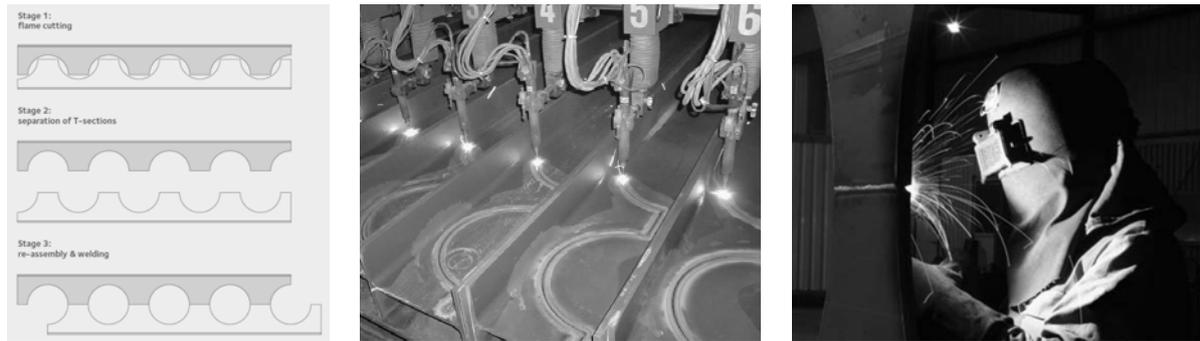
Figure 1: Fabrication process a) Principle – b) Flame cutting – c) Welding of webs
