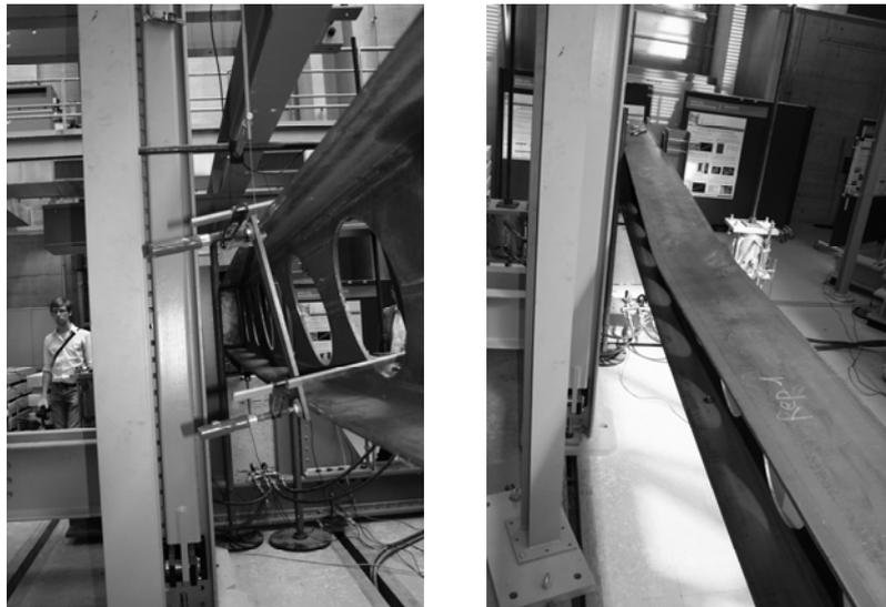
Figure 15: a) Lateral torsional deformed configuration at failure – b) Residual deformation after unloading
