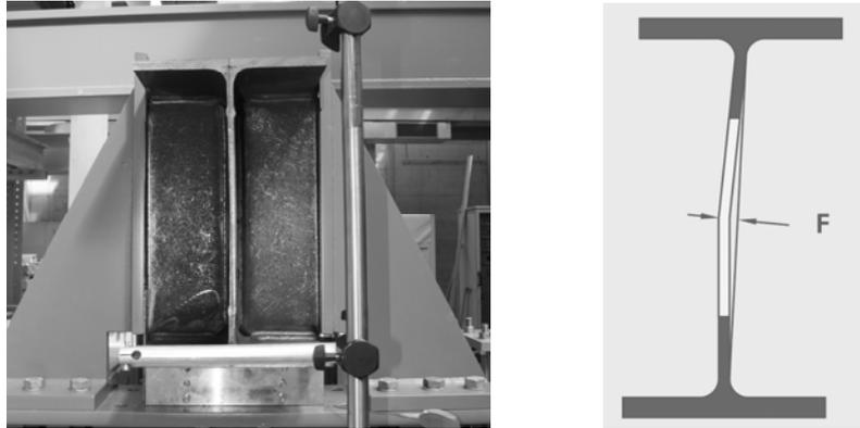
Figure 9: “Bending of web” initial cross-sectional imperfection
