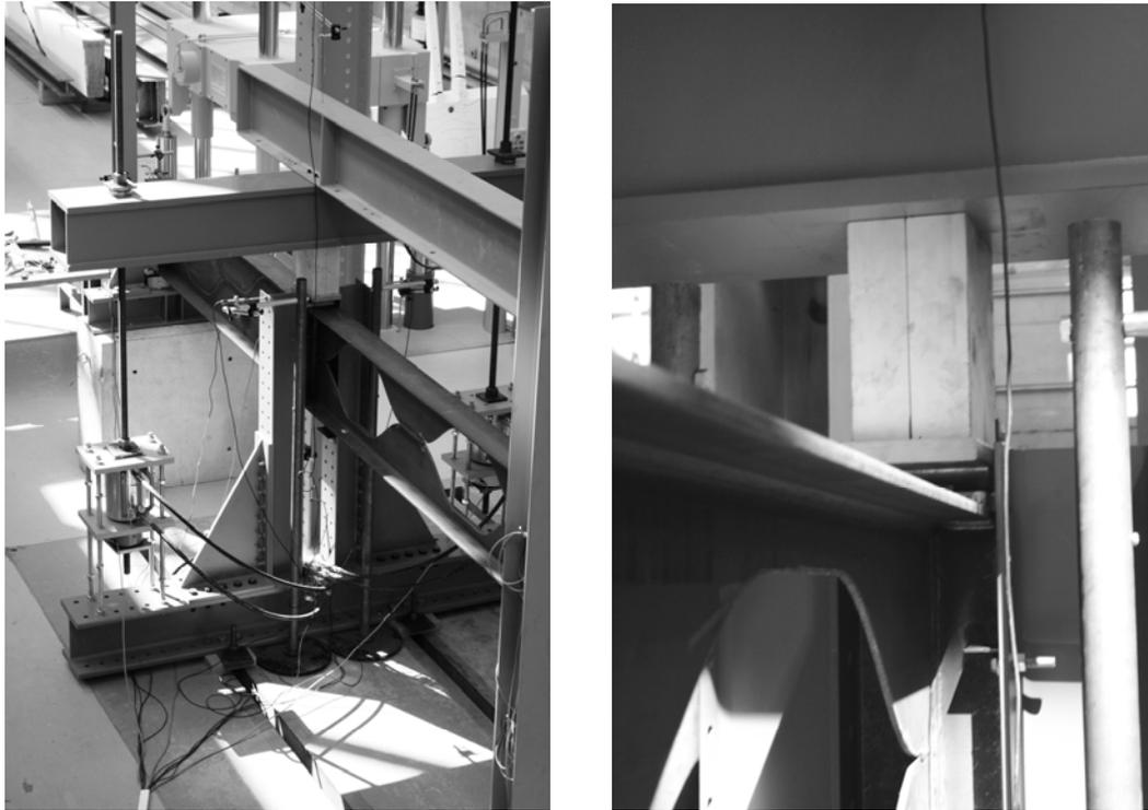
Figure 6: Rigid girder and roller support for load introduction
