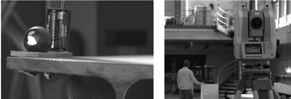
Figure 11: Measurement of flanges' edges a) Trolley and light – b) optical measure
