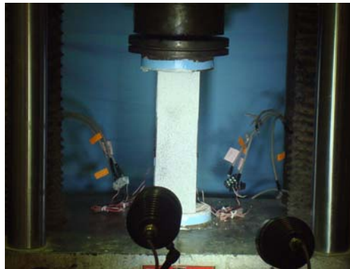
Figure 5: Stub column test setup
