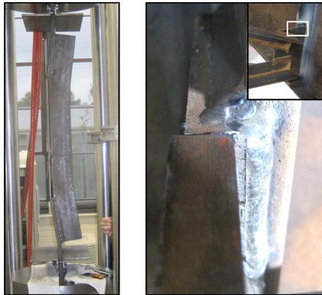
Figure 4: (a) Single angle member yielded in tension and (b) Out-of-plane movement of cracked gusset plate with stiffener shown
