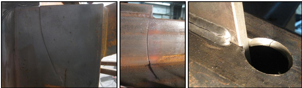
Figure 12: Fatigue cracks at failure for (a) X frame, (b) K frame, and (c) Z frame
