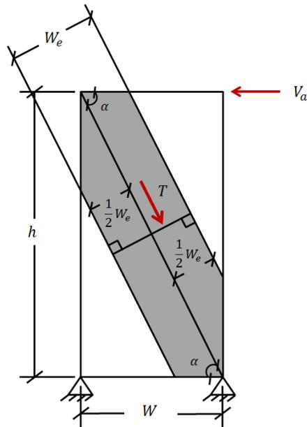
Figure 5: Effective strip model of steel sheet sheathing
