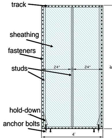
Figure 1: Components in a typical CFS shear wall
