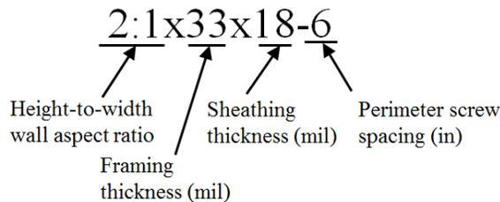
Figure 12: Definition of shear wall configuration
