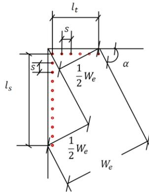
Figure 7: Sheathing-to-framing fastener connection layout within effective strip
