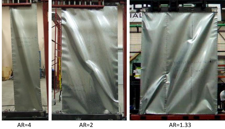
Figure 4: Tension field action of CFS-SSSWs
