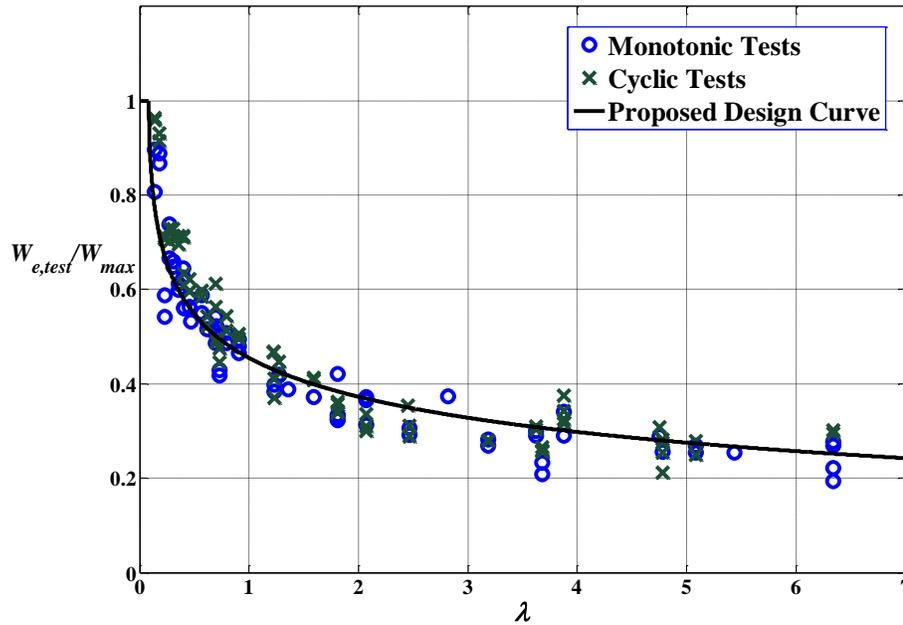
Figure 9: Comparison between the proposed design curve with test results
