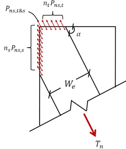
Figure 6: Equilibrium of nominal tension force in sheathing and sum of nominal connection shear capacity
