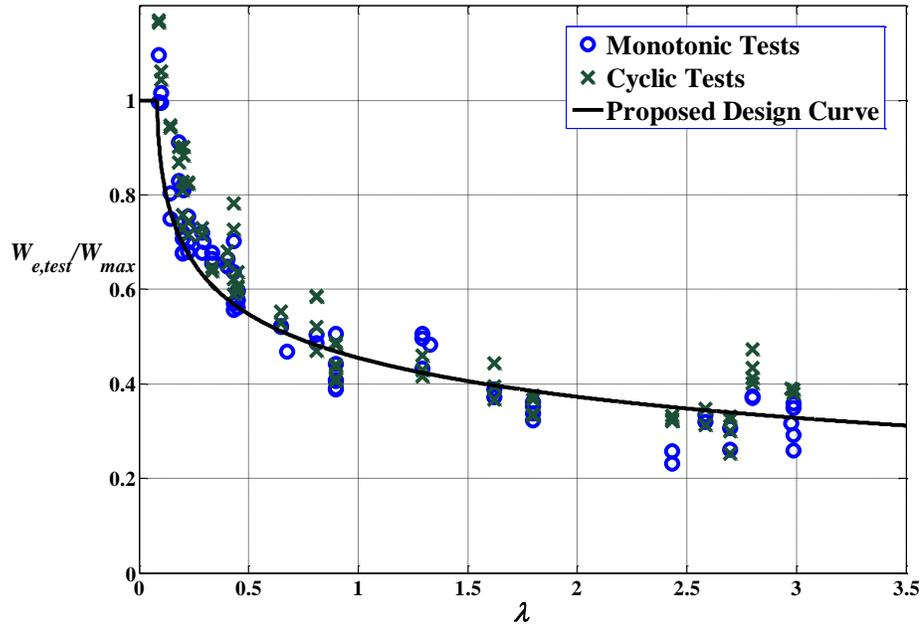
Figure 10: Comparison between the proposed design curve with test results (Nominal)
