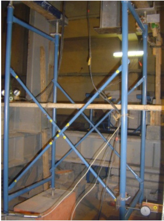
Figure 2: Tested scaffolds: Cuplock - Wedge type - Braced frame - Braced frame with tie
