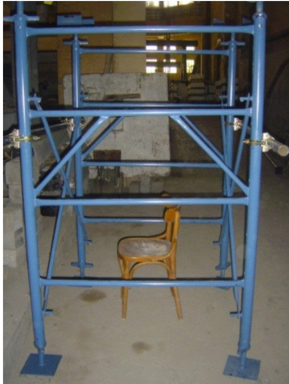
Figure 2: Tested scaffolds: Cuplock - Wedge type - Braced frame - Braced frame with tie
