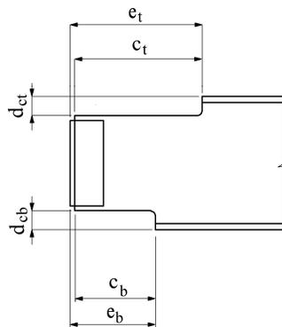
Figure 2. Different Cope Sizes at the Top and Bottom Flanges
