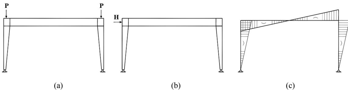
Figure 2: Tapered hinged base frame: (a) column load, (b) horizontal unit load, (c) corresponding bending moment
