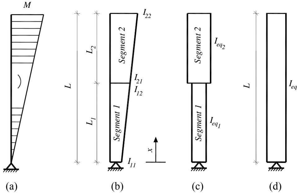
Figure 5: Converting a two segment tapered column to an equivalent prismatic column
