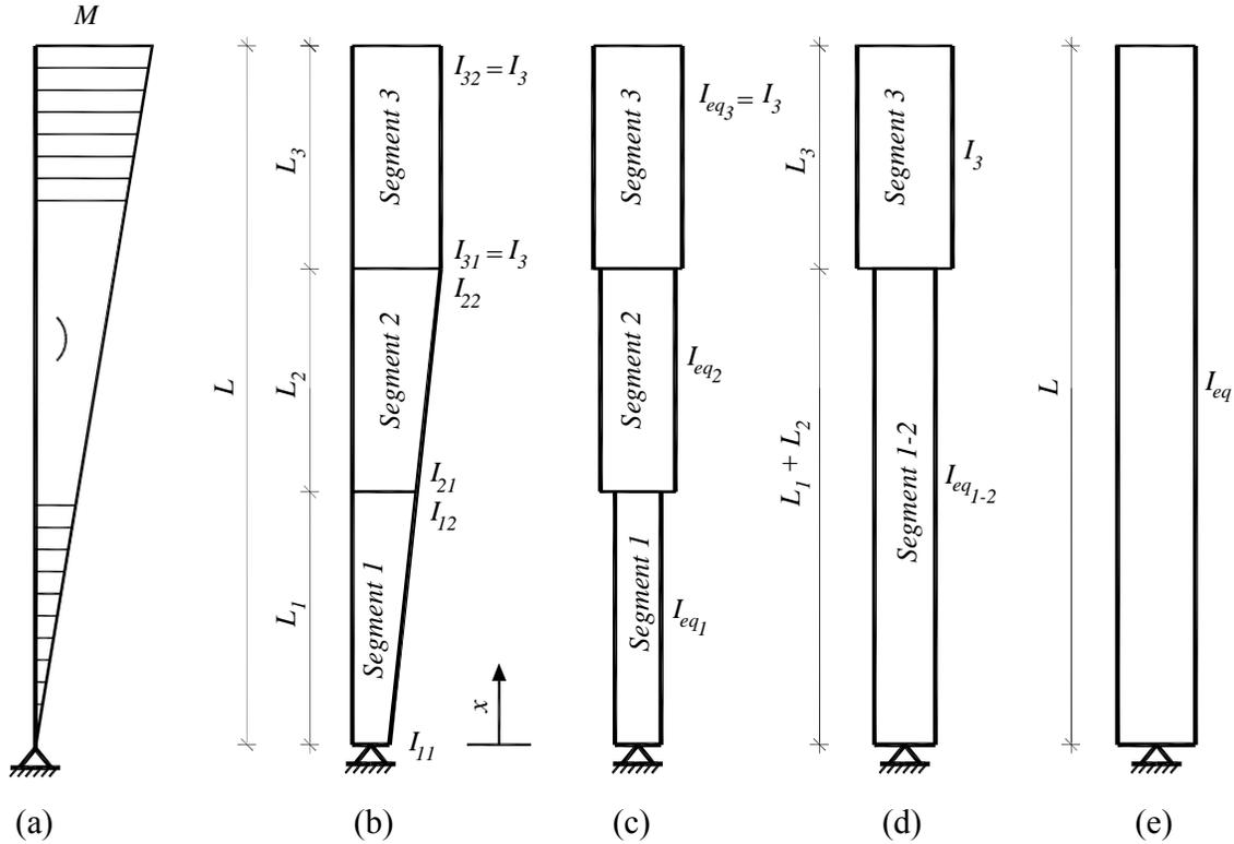
Figure 7: Converting a tapered-constant column to an equivalent prismatic column
