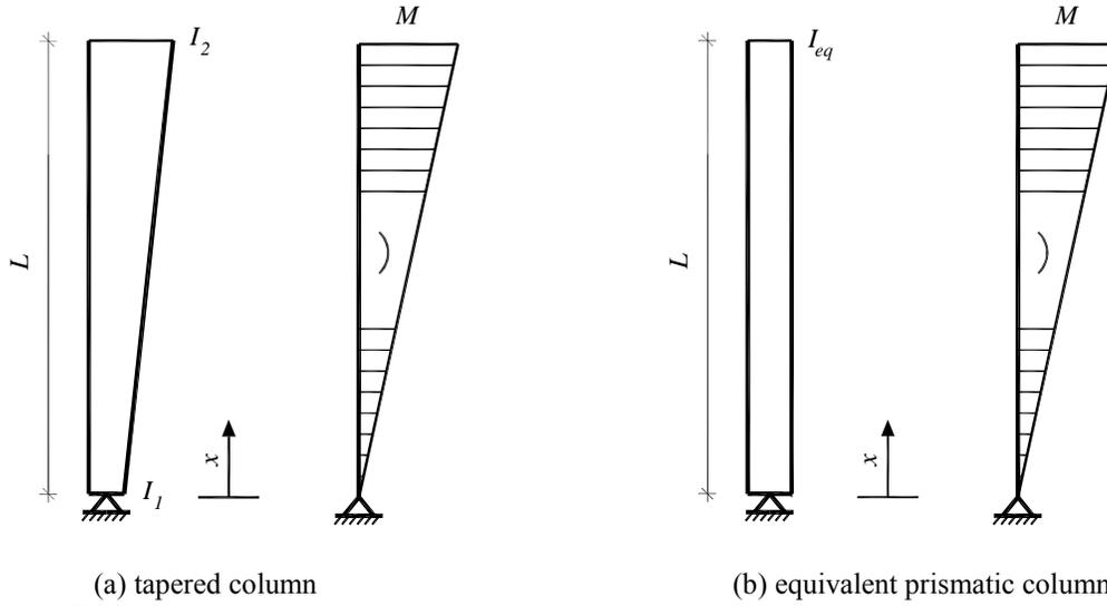
Figure 3: Tapered and equivalent prismatic column in sway frame with corresponding bending moments
