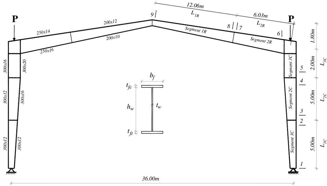
Figure 10: Frame geometry and loads (Example 4)
