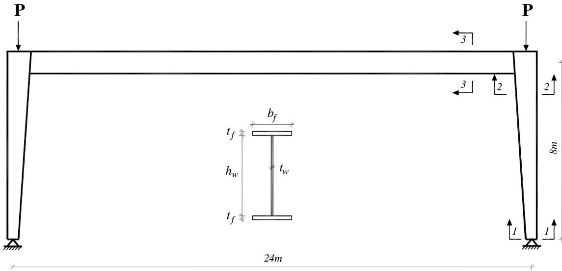
Figure 8: Frame geometry and loads (Examples 1 and 2)
