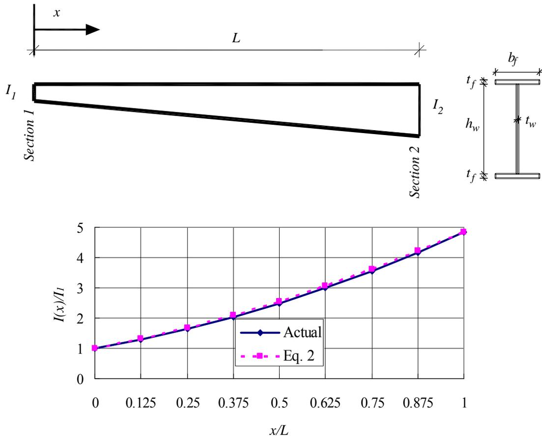
Figure 1: Comparison between actual moment of inertia and moment of inertia calculated using Eq.2
