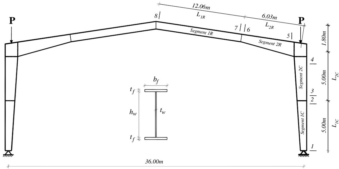
Figure 9: Frame geometry and loads (Example 3)
