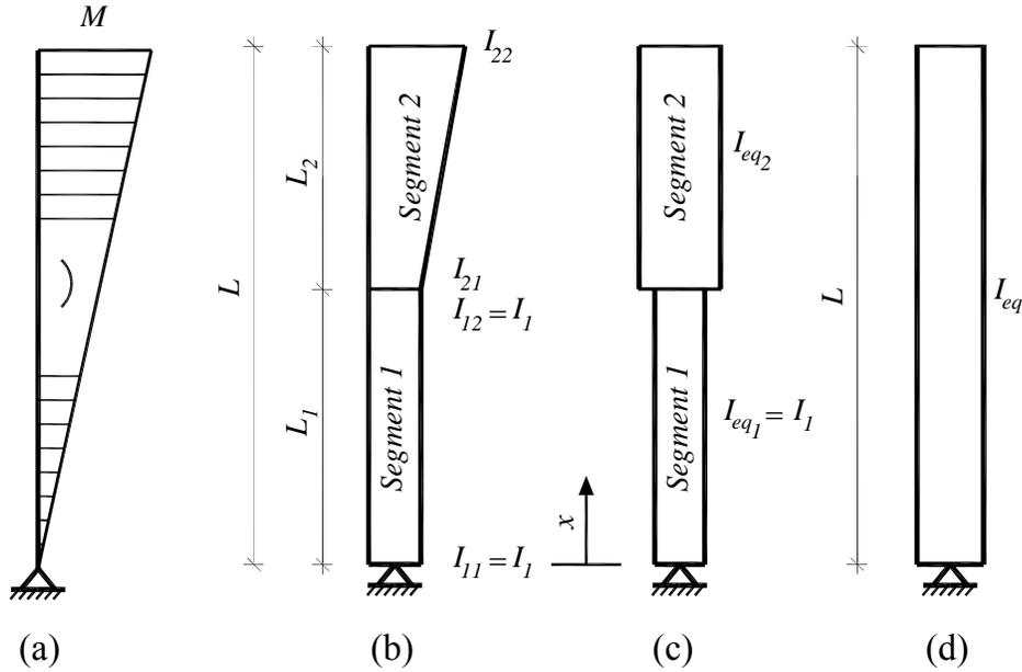
Figure 6: Converting a constant-tapered column to an equivalent prismatic column
