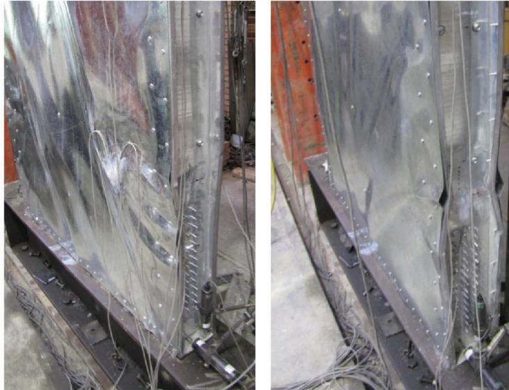
Figure 8: Failure modes for 1.2F-0.8Sh-0F specimen (left) and 1.2F-0.8Sh-BF specimen (right)
