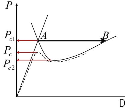
Figure 1: Load-deformation for perfect and imperfect shell structure
