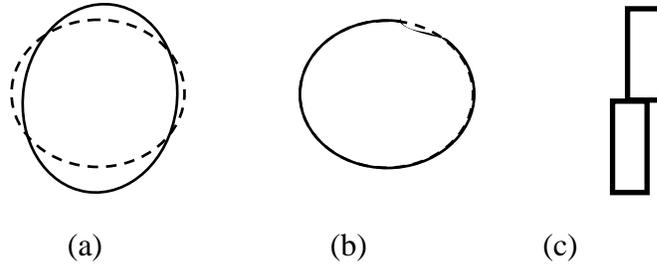
Figure 2: Imperfection types considered in Eurocode buckling quality class calculations: (a) Out-of-Roundness (b) Dimple (c) Accidental Eccentricity
