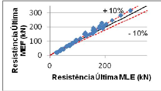
Figure 3: Comparison for the ultimate resistance results obtained via MLE and MEF at 20° C.
