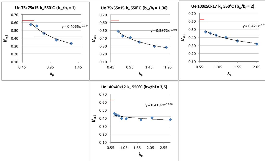
Figure 5:  $k'_{\sigma,\theta}$  coefficient variation in relation to the relative slenderness separated in  $b_w / b_f$  ratio groups at a temperature of 500 °C.
