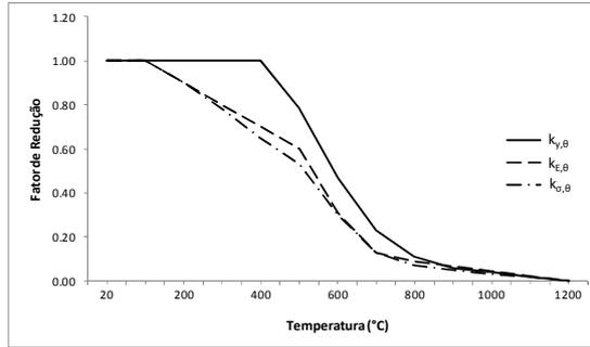
Figure 1: Variation of reduction factors  $k_{y,\theta}$ ,  $k_{\sigma,\theta}$  and  $k_{E,\theta}$  as a function of steel temperature (EN 1993-1-2:2005)
