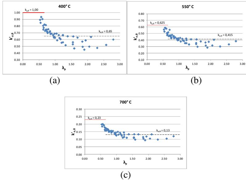
Figure 4: Variation of the theoretical  $k'_{\sigma,\theta}$  reduction factor as a function to the cross-section relative slenderness in high temperatures: (a) 400° C, (b) 550° C (c) 700° C.
