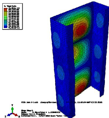
Figure 2: Local Buckling Mode
