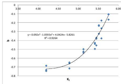
Figure 7: Variation of b coefficient in relation to the  $k_l$  coefficient
