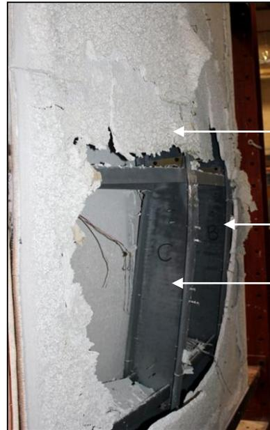
(b) Partial fall-off of fire side plasterboards
