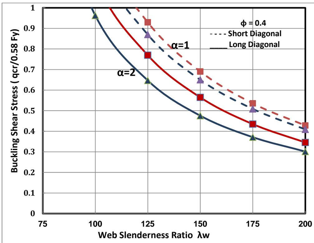
Figure 3: Variation of Shear Buckling Stress according to Compression Diagonal Direction
