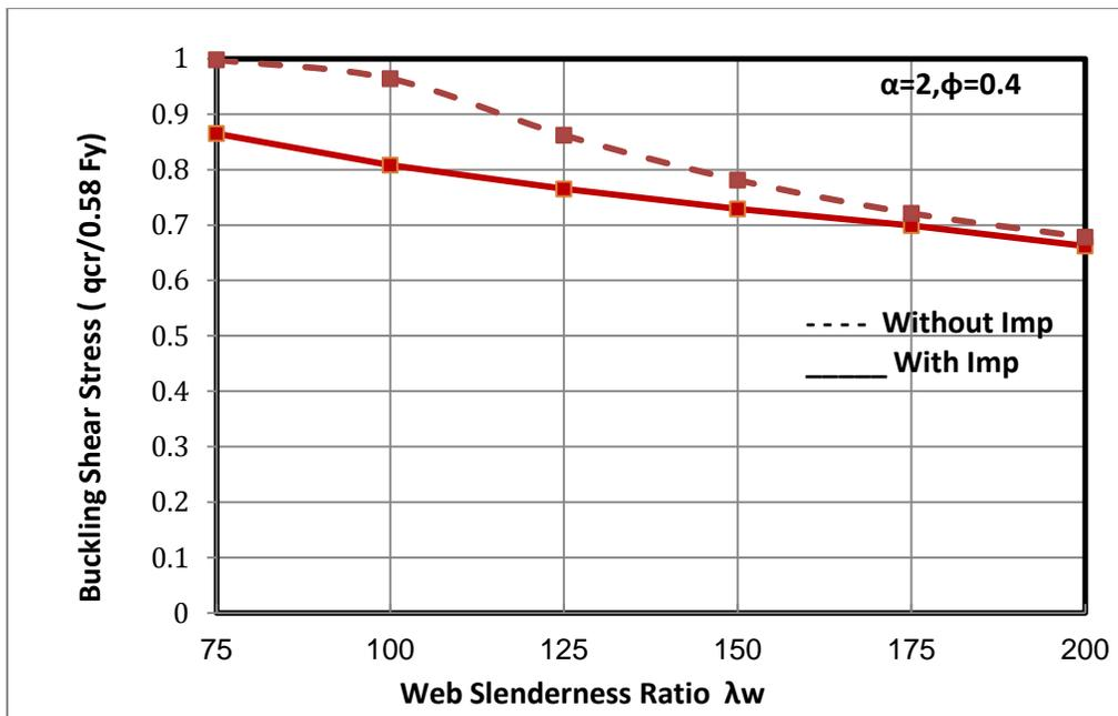
Figure 6: Reduction in Ultimate Shear Stress due to Imperfections ( $\alpha=2$ ,  $\text{tgt } \phi=0.2, 0.4$ )
