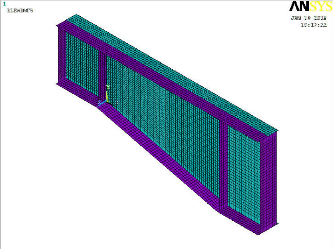
**Figure 2: Finite Element Model**
