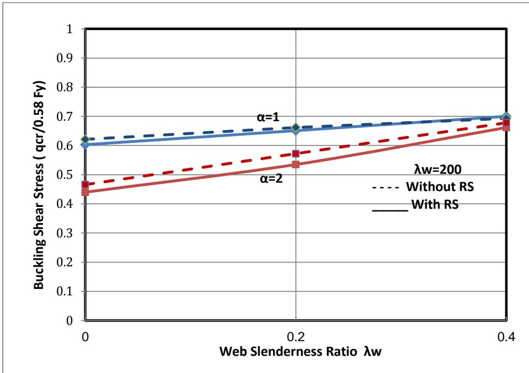
**Figure 7: Reduction in Ultimate Shear Stress due to Imperfections for different  $\alpha$  and  $\phi$  values**
