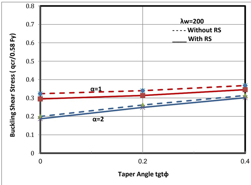
**Figure 5: Reduction in Shear Buckling Stress due to Residual Stresses for different  $\alpha$  and  $\phi$  values**
