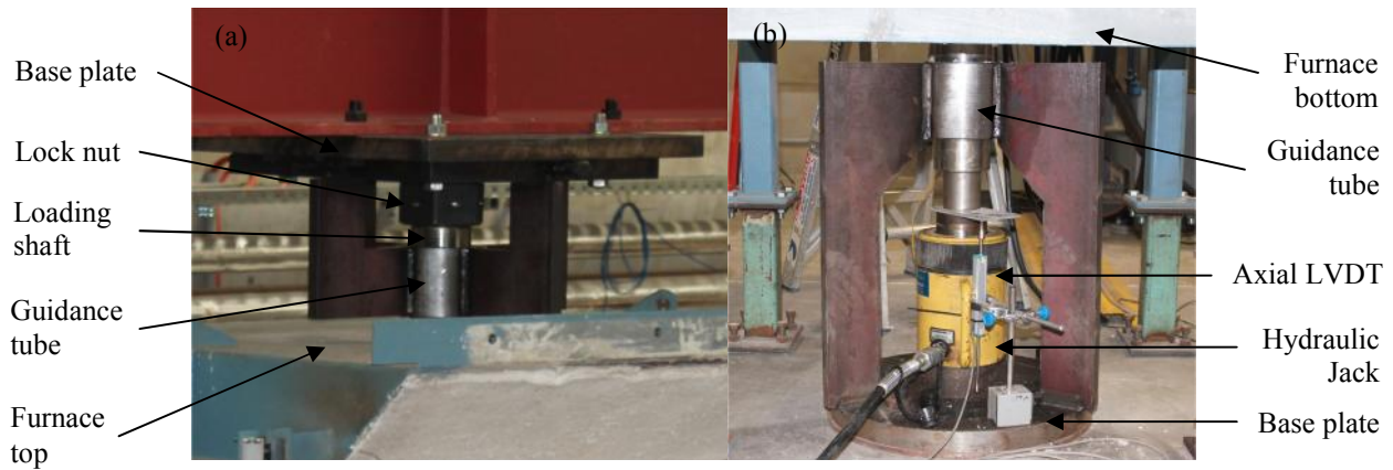
Figure 2: (a) Top loading arrangement (b) Bottom loading arrangement
