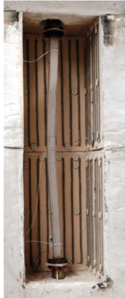
Figure 3: Typical failure of tested columns
