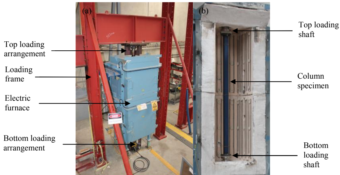
Figure 1: (a) Overall test set-up (b) Test column
