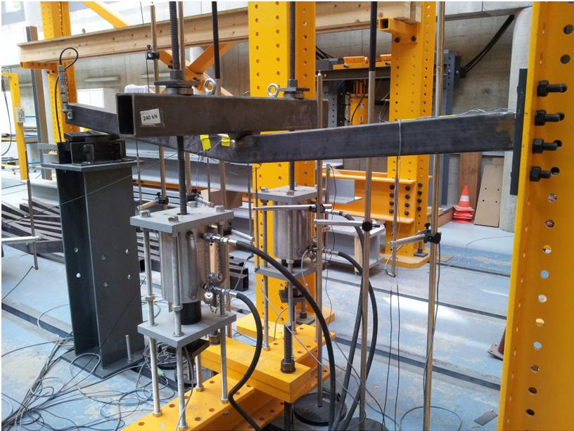
Figure 19: Propped cantilever after testing
