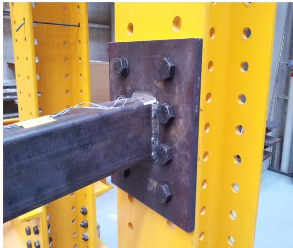
Figure 18: Frame to beam fixed end connection
