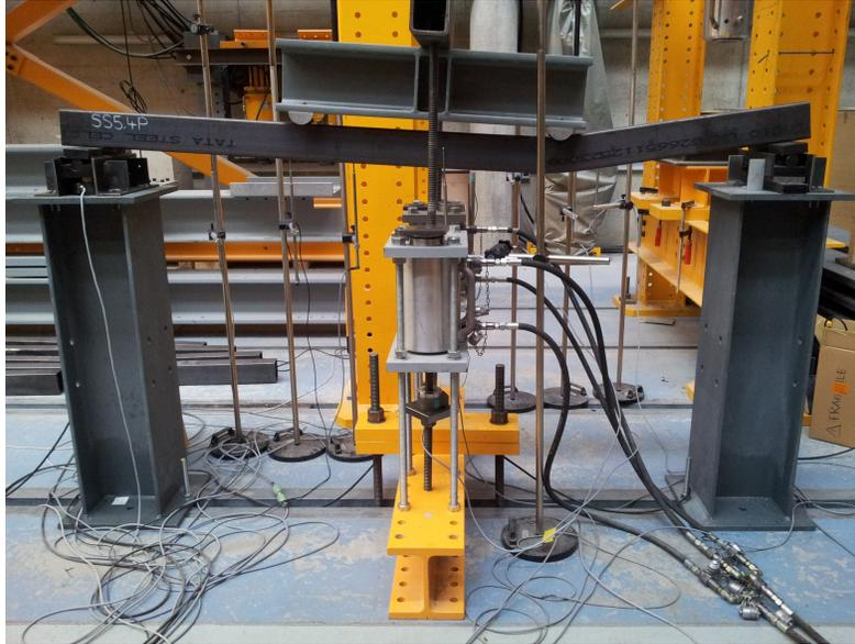
Figure 7: Post-test deformed shape of beam SS5.4P
