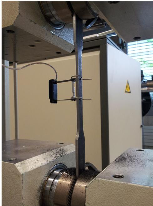
Figure 1: Tensile coupon specimen and attached clip gauge
