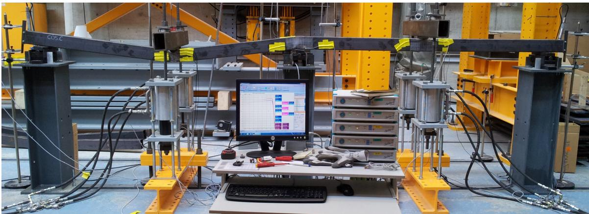
Figure 10: Deformed shape of continuous beam CO5.C after testing
