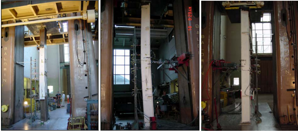
Figure 7: Column and beam-column tests setup (Left: single-rib column test, Middle: single-rib beam-column test, Right: triple-rib beam-column test)
