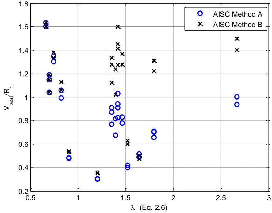
Figure 2.6: Comparison of shear test results with AISC design methods
