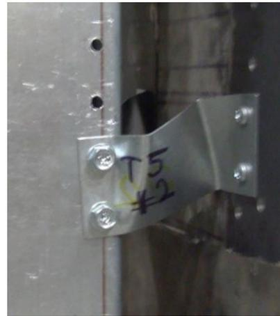
Figure 2.3: Test result of clip angle T5a#2
