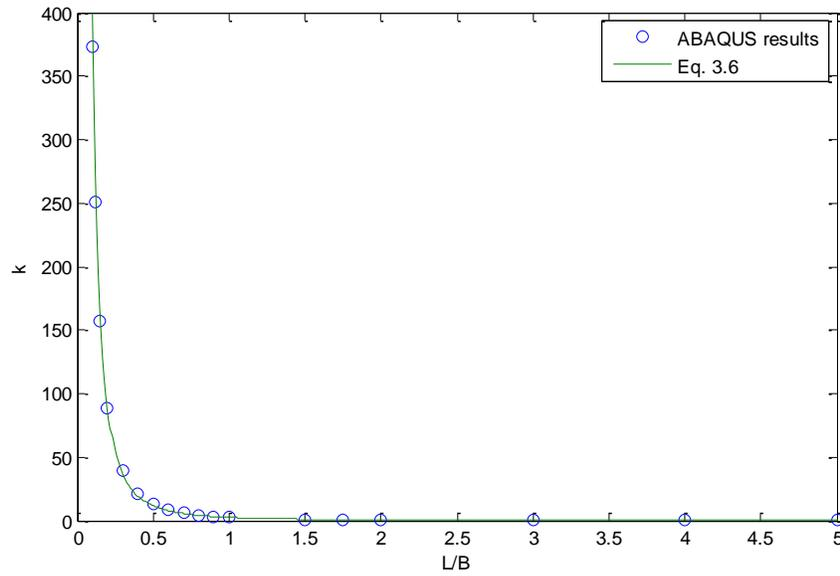
Figure 3.4: Comparison of buckling coefficient, k
