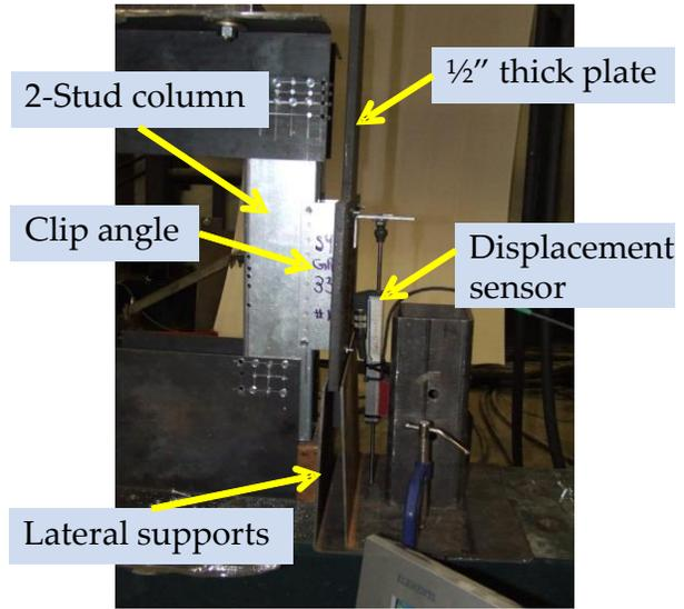
Figure 2.2: Close-up view of shear test setup
