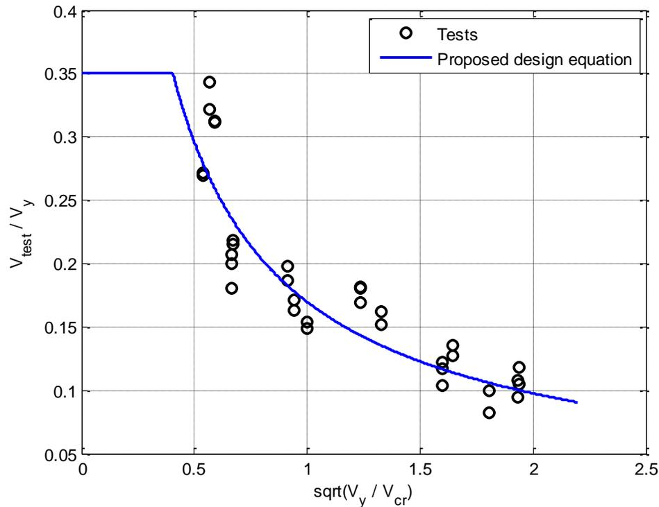
Figure 3.1: Comparison of shear test results with proposed design method
