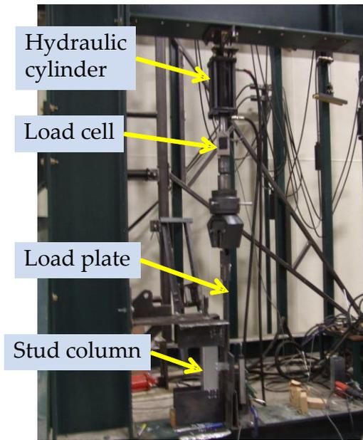
Figure 2.1: Overall view of shear test setup
