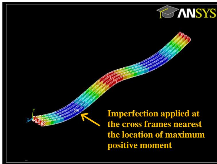
Figure 3: Static Analysis of Two-Span Continuous Bridge to Identify Location of Maximum Moment
