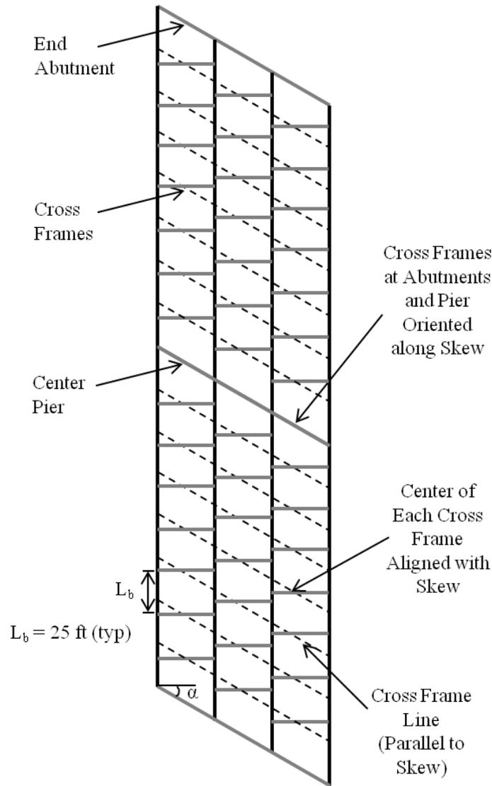
Figure 5: Bridge Layout Used in Study
