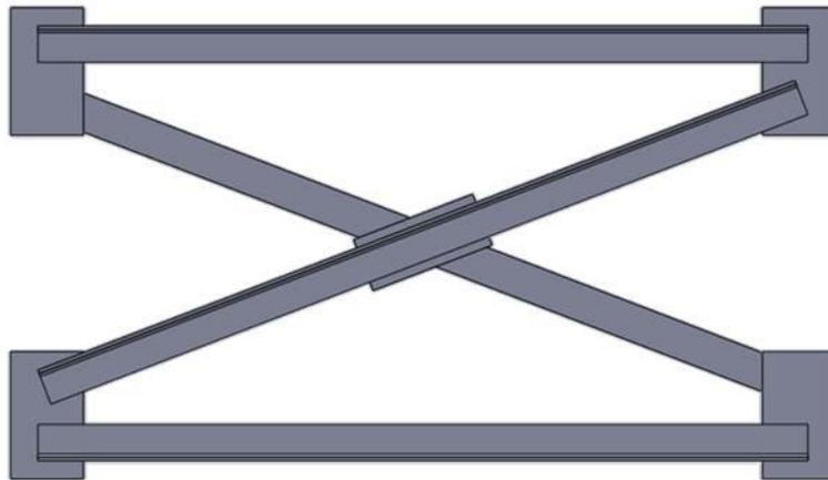
Figure 1: Typical X-Type Cross Frame with Steel Angles
