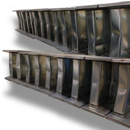
Figure 5: All tested specimens: Buckling shape of the specimens
