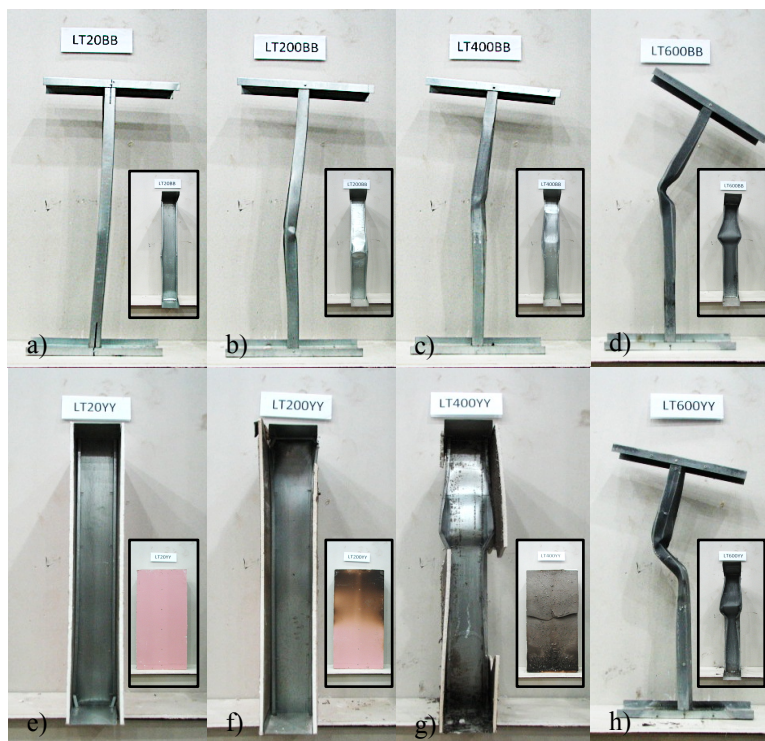
Figure 8: 1.0 m long specimens after testing: bare studs tested at a) 20°C, b) 200°C, c) 400°C and d) 600°C, and studs sheathed with fire-rated gypsum tested at e) 20°C, f) 200°C, g) 400°C and h) 600°C
