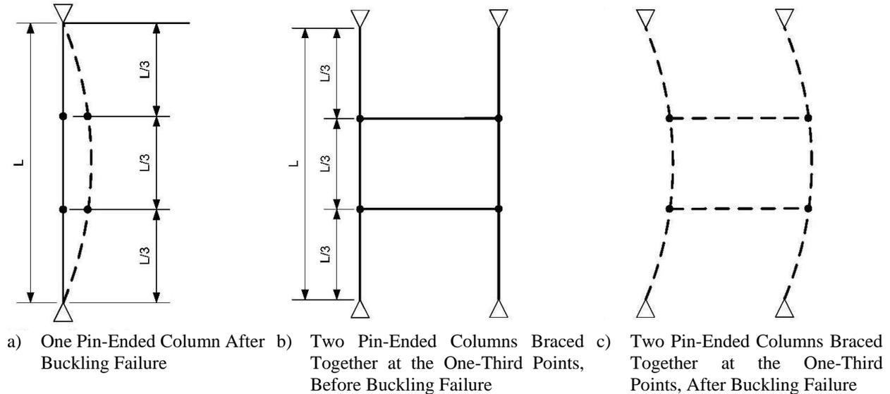
Figure 6. Pin-Ended Column Example Showing Overall Buckling of a) Single Pin-Ended Column; b) Two Pin-Ended Columns with c) Ineffective Bracings
