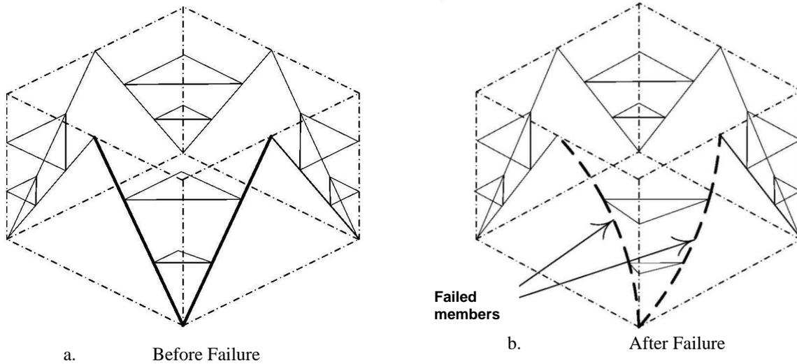
Figure 13. General Isometric View, a) Typical Vertical and Horizontal Column Bracing Configuration, b) Showing Buckled Vertical Braces Unrestrained by the Horizontal Bracings
