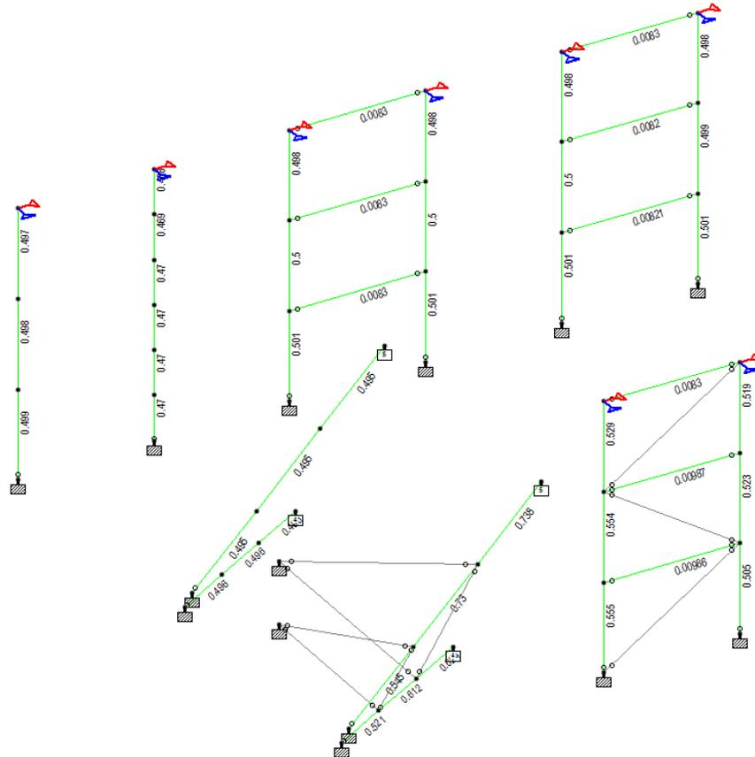
Figure 9. STAAD Pro Direct Analysis Method Results Showing Unity Ratio Checks
