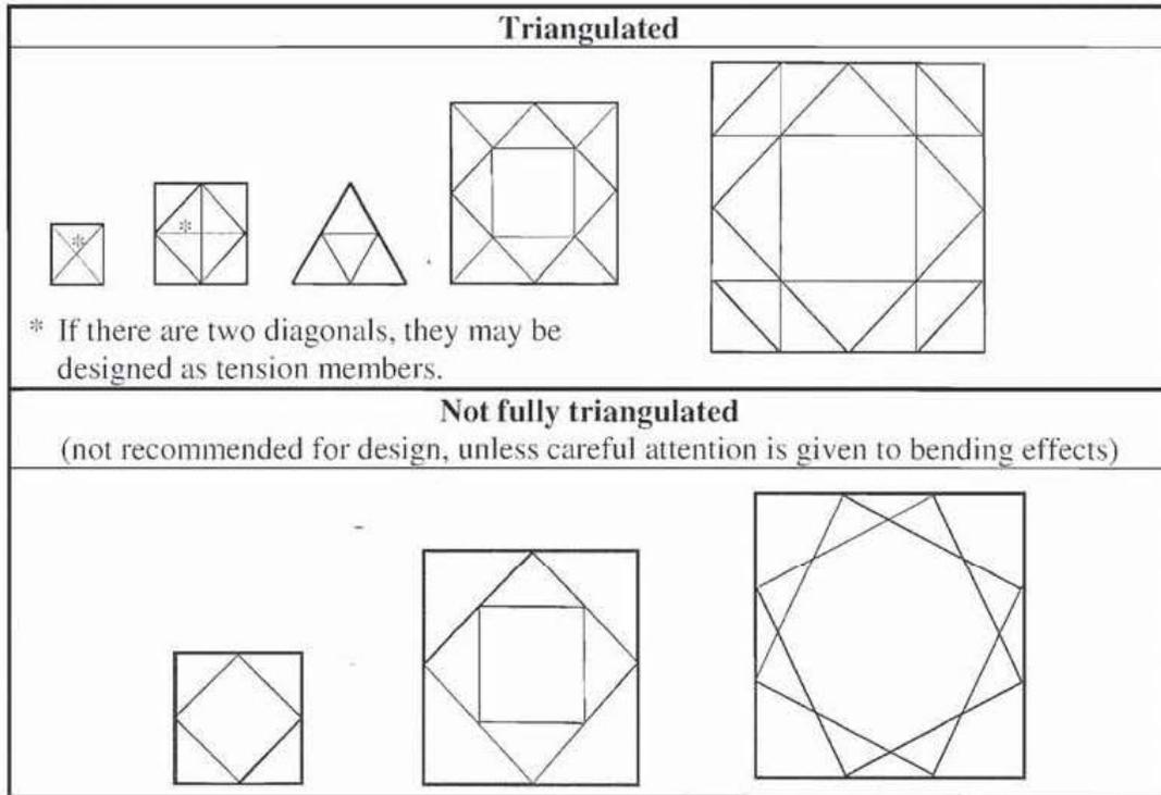
Figure 4. Typical Plan Bracing (EN 1993-3-1:2006)
