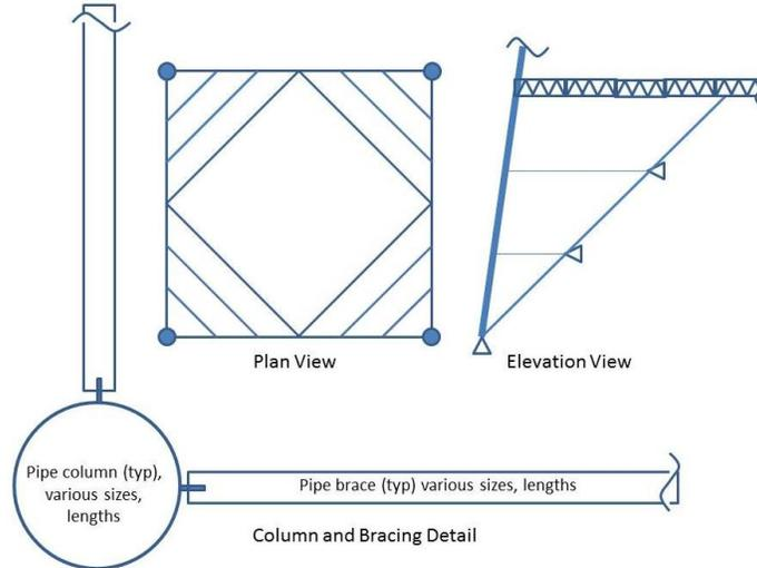
Figure 11. General Column and Bracing Detail, Plan and Elevation Views
