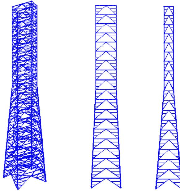
Figure 1. Flare Derrick Structure - Overall View STAAD Pro Model
