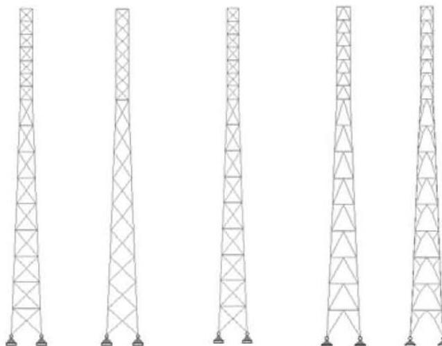
Figure 2. Models of 164 ft. (50m) Towers with different Bracing Systems (Jesumi and Rajendran, 2013)
