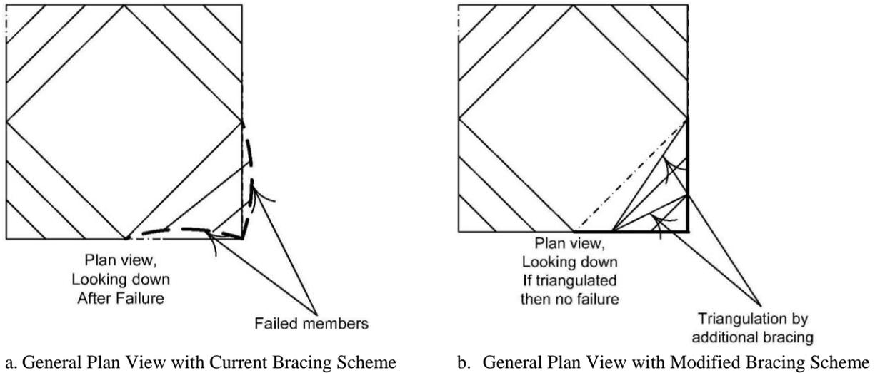
Figure 12. General Plan View of Vertical and Horizontal Bracing, a) Showing One Leg with Buckled Vertical Braces, and b) Proposed Bracing Members Added to Prevent Buckling Mode as Illustrated in a).
