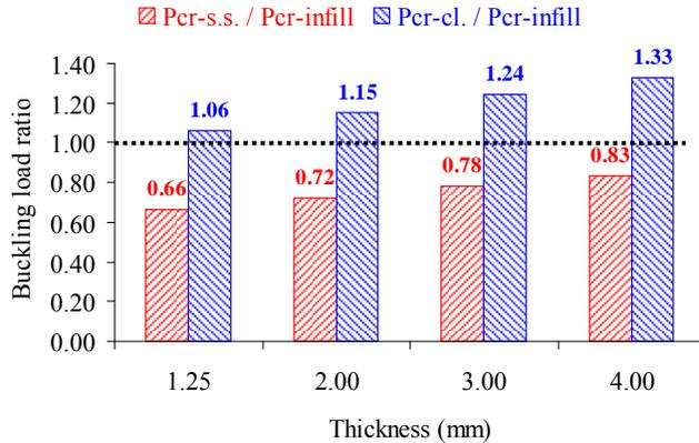
Figure 7: Plate-frame interaction in buckling of SPSWs with flat infill plates
