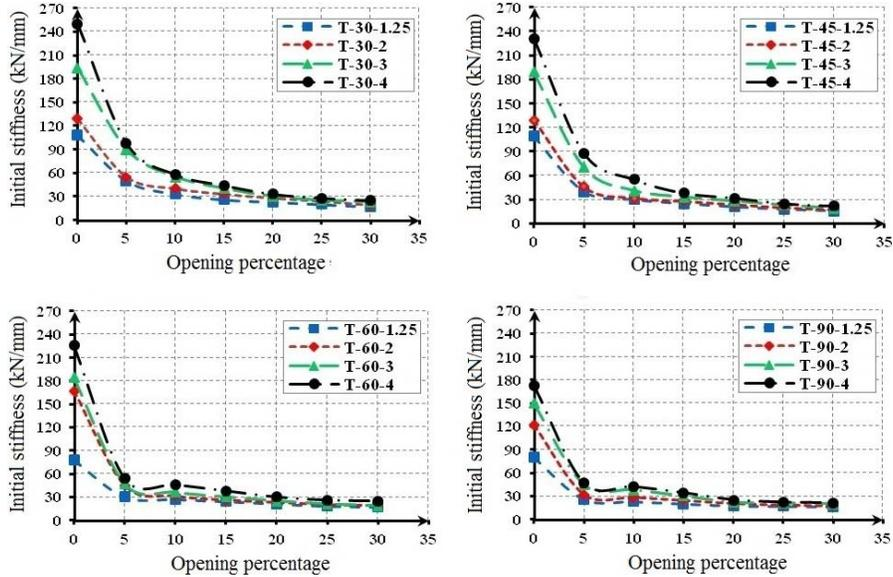
Figure 9: Initial stiffnesses of the SPSW models with 30°, 45°, 60°, and 90° corrugation angles
