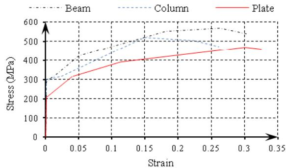
Figure 4: Stress-strain relationships of the steel material (Emami and Mofid, 2014)
