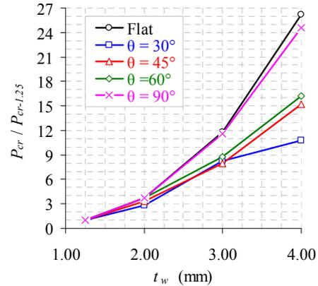
Figure 8: Variation of buckling strength of SPSWs with non-perforated infill plates
