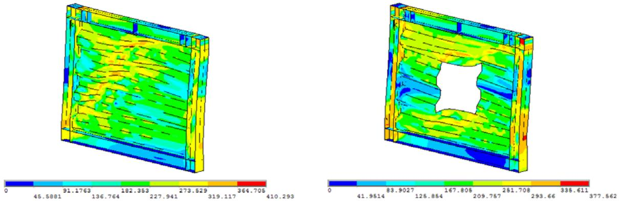
Figure 10: von Mises stress contour plots of  $T-45-3-0$  and  $T-45-3-15$  models
