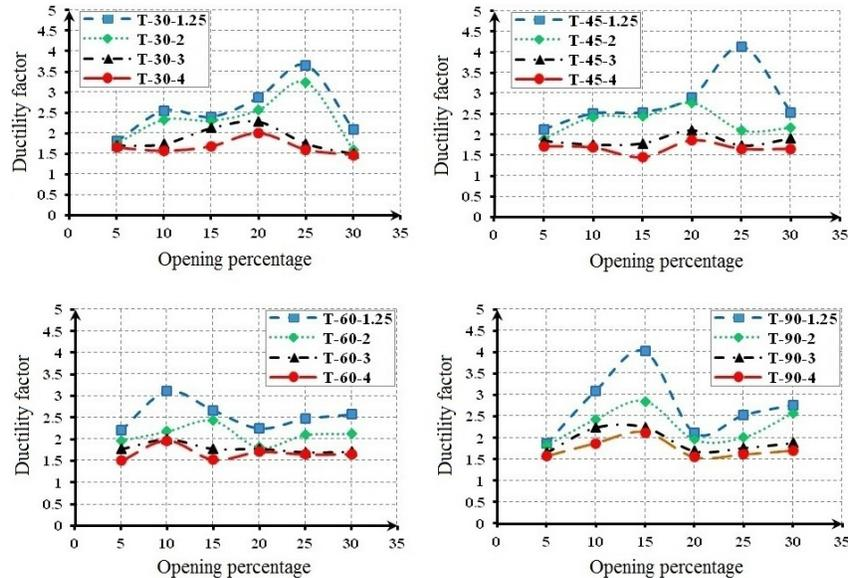
Figure 12: Ductility of the SPSW models with 30°, 45°, 60°, and 90° corrugation angles
