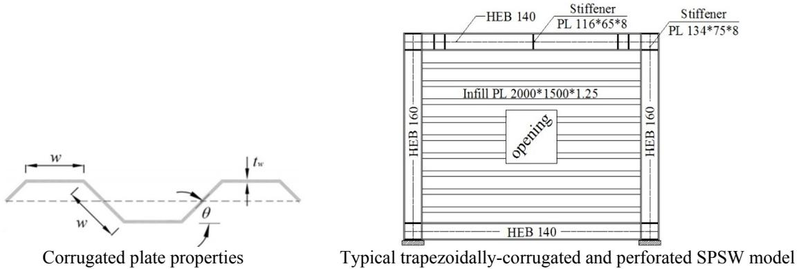
Figure 2: Geometrical properties of considered SPSW models
