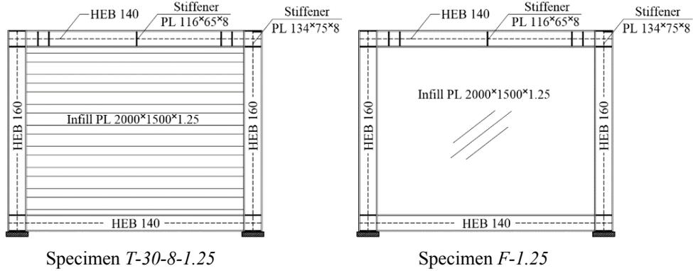
Figure 1: Details of the modeled experimental specimens tested by Emami et al. (2013)
