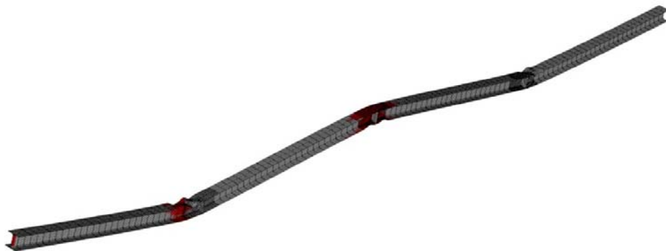
Figure 30: Typical plastic failure mode for case 3 configuration (yield pattern, HEB section)
