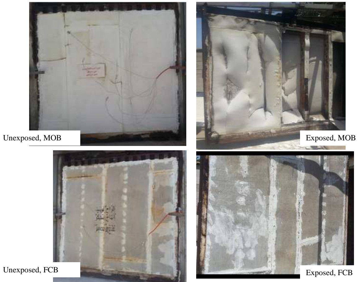
Figure 3: Exposed and unexposed surfaces of walls after fire test
