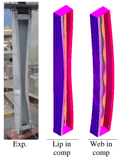
Figure 11: Load-horizontal displacements of web central point and modes of failure of specimen L120 (pre-fire)
