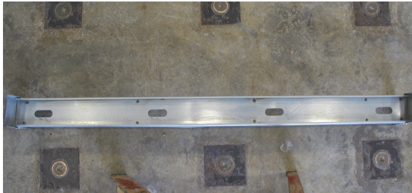
Figure 6. Typical Screw Spacing and Layout
