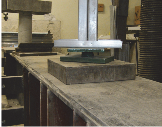
Figure 4. Bottom Pin Connection
