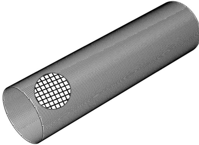
Figure 3: Mesh layout for Specimen SW-325-120° with detail showing mesh oriented at 6° angle of inclination.
