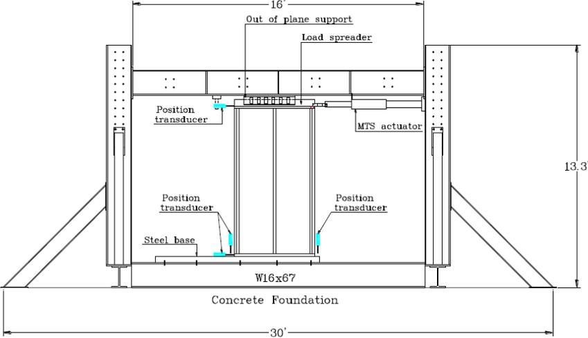
Figure 1: Shear Wall Testing Frame
