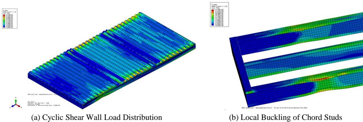
Figure 12: ABAQUS Deformation Response
