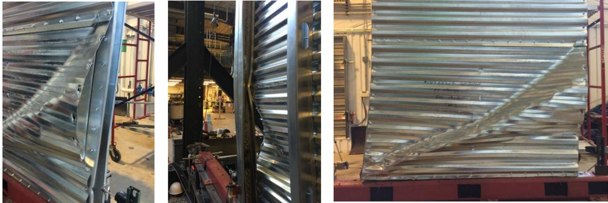
(a) Screw Pull Over      (b) Local and Torsional Buckling      (c) Shear Buckling
