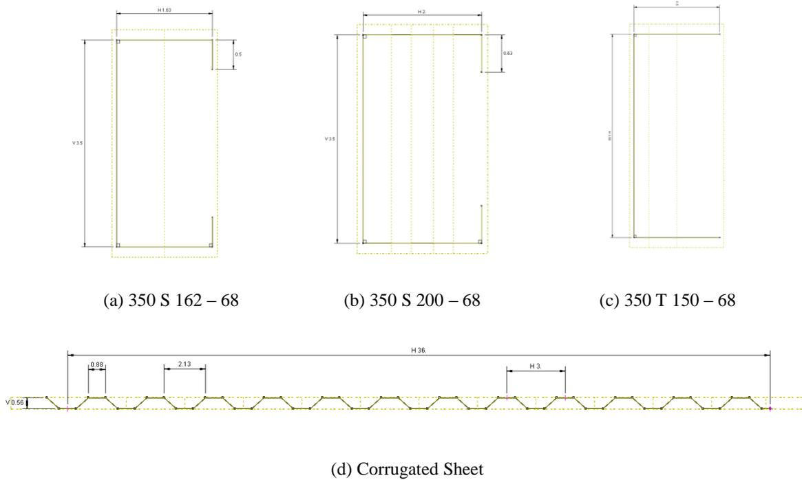
Figure 7: Cross Sectional Geometry of Shear Wall Components
