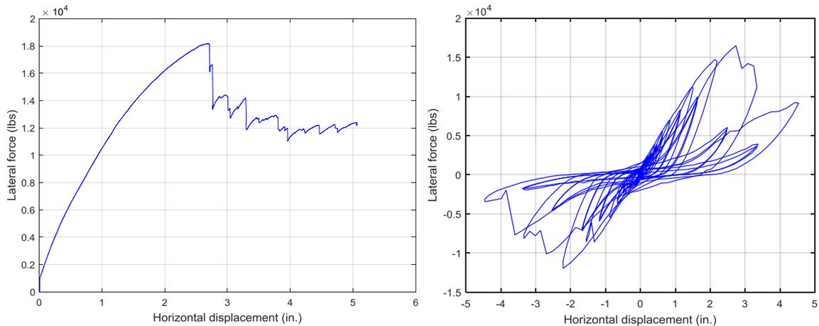
Figure 4: Load-Deformation Response of Monotonic and Cyclic Test
