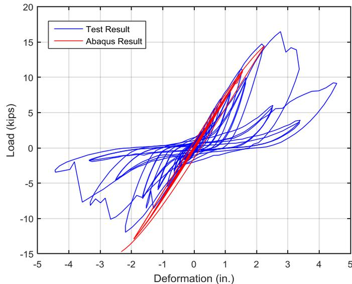
Figure 13: Load-Deformation Response Comparison
