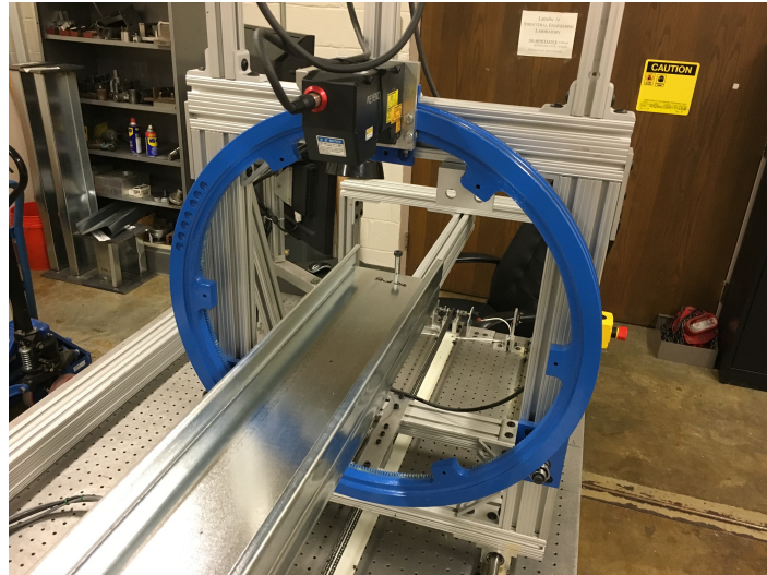
Figure 8: Laser scanner setup with built-up specimen installed
