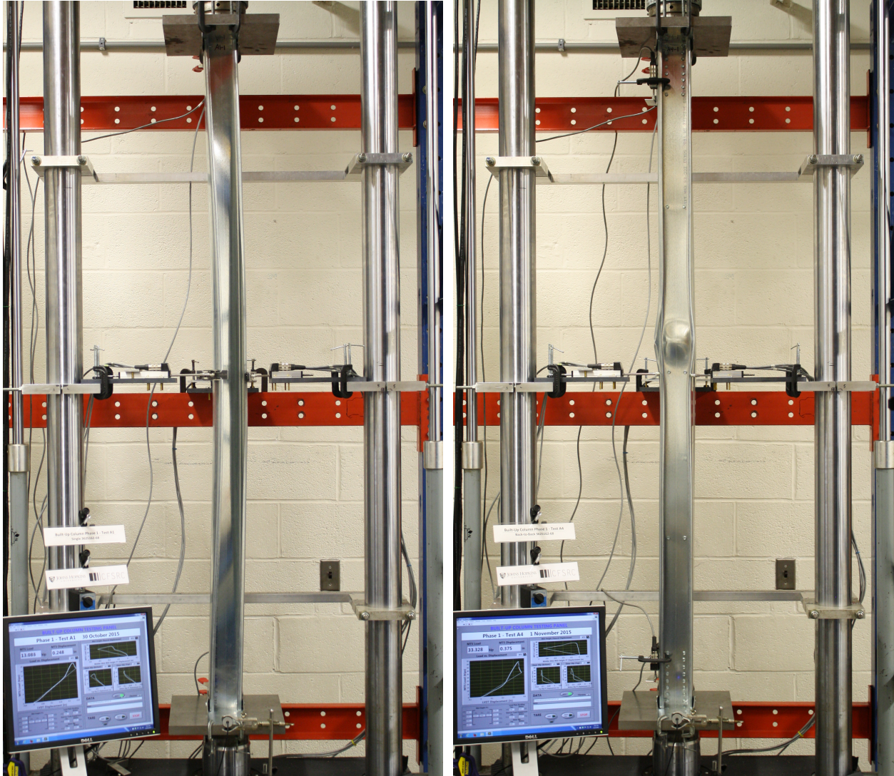
Figure 13: Typical flexural-torsional (left, trial A1) and interacting local/flexural (right, trial A4) buckling failures
