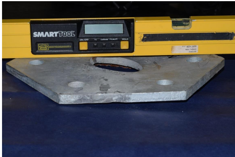
Figure 7: Permanently deformed plate between weldments
