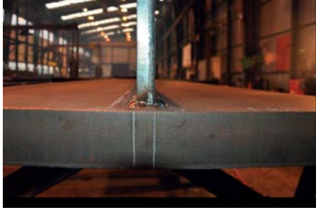
Figure 6: Experimental division of flange into strips (flame-cut specimen with width of 730 mm)
