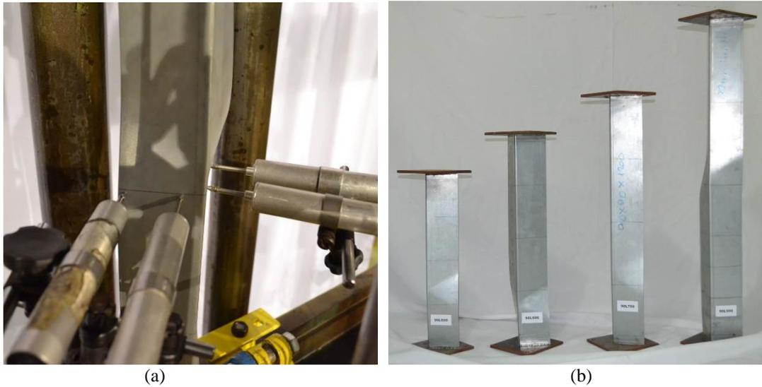
**Figure 15:** (a) Close view of the most deformed region of specimen 600L900 just after collapse and (b) joint view of the specimens belonging to the 90 series after the load removal.
