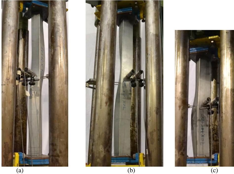
**Figure 14:** Deformed configurations at the onset of collapse of specimens (a) 600L900, (b) 700L900 and (c) 700L600.
