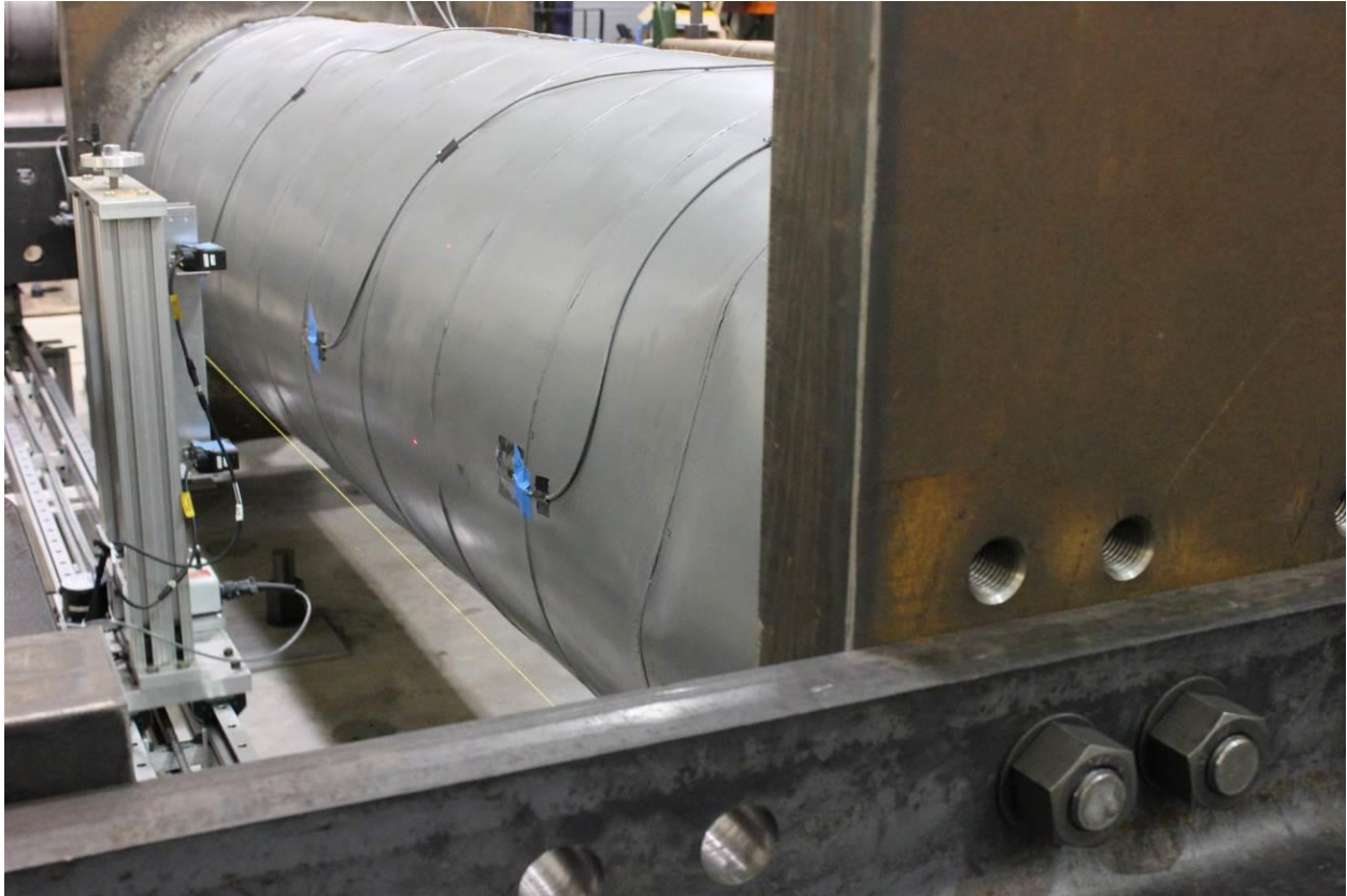
Figure 8: Image showing the laser scanning rig (towards the left of the figure) used to measure deformation during testing.
