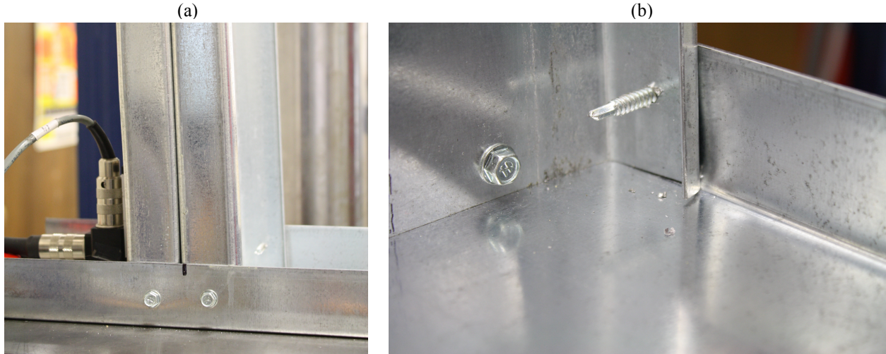
Figure 13. Side view of (a) a semi-rigid condition at peak load and (b) corresponding lip/flange lift-off for C2-54
