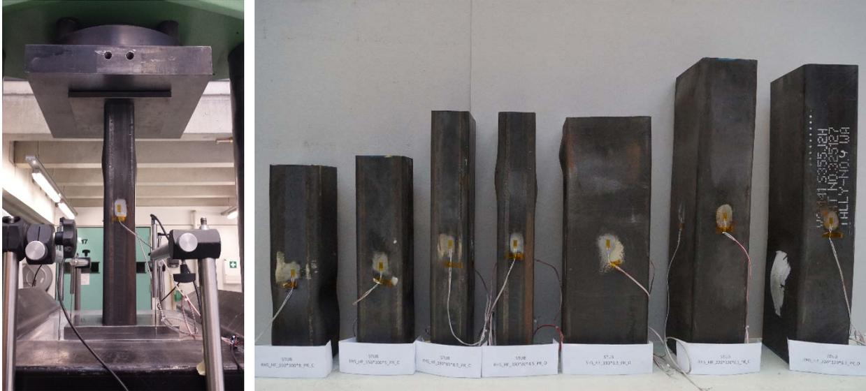
Figure 5 – Testing and failure shapes of stub columns
