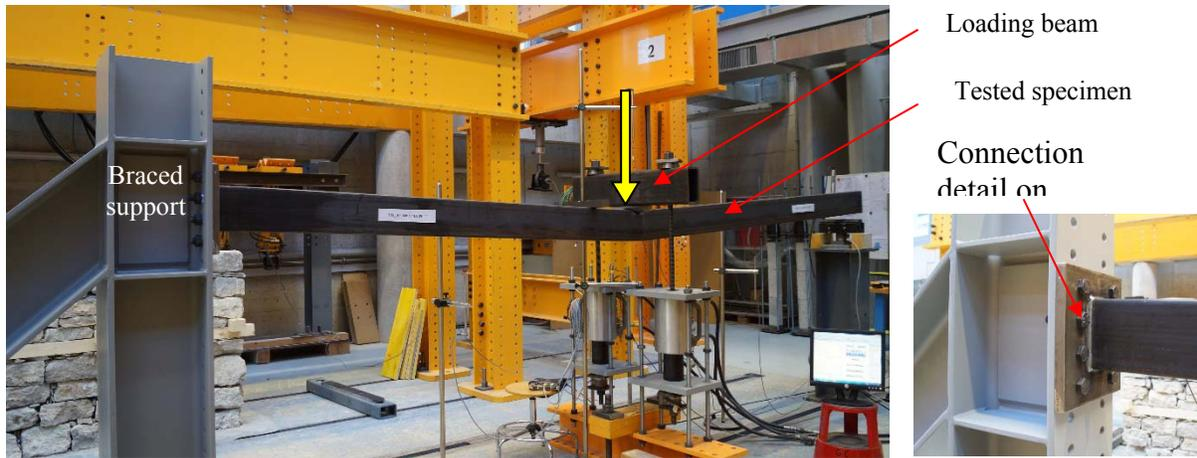
Figure 13 – a) Deformed shape of a propped-cantilever centrally loaded – b) Connection detail on braced support
