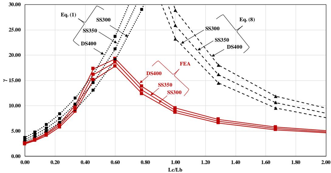
Figure 6: Buckling load predictions for the systems with  $L = 50\text{m}$
