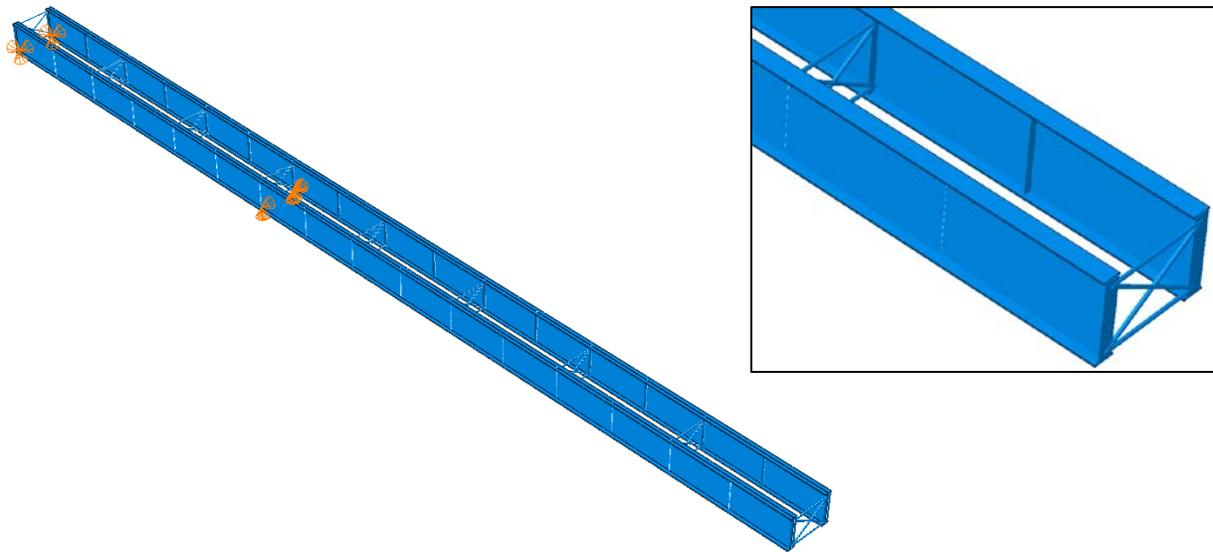
Figure 3: Three-dimensional representation of a typical girder system modeled in the ABAQUS program
