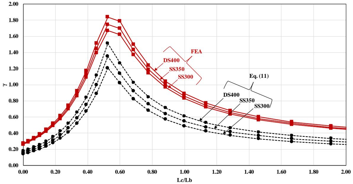
Figure 11: Buckling load predictions for the systems with  $L = 100\text{m}$  obtained with the proposed method
