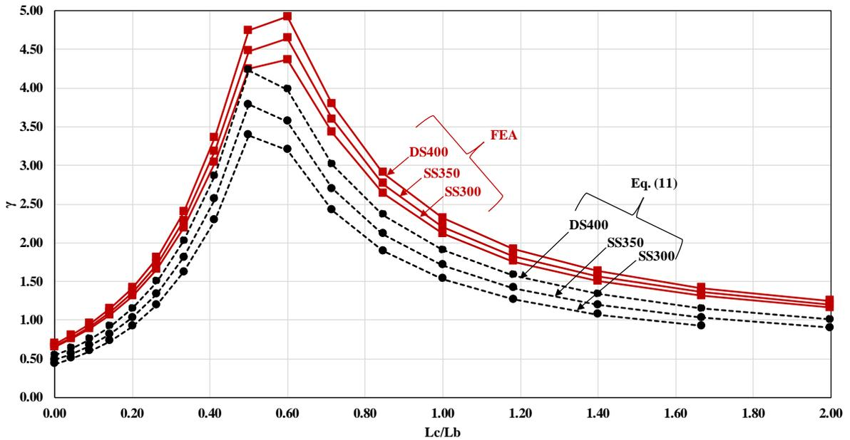
Figure 10: Buckling load predictions for the systems with  $L = 75\text{m}$  obtained with the proposed method
