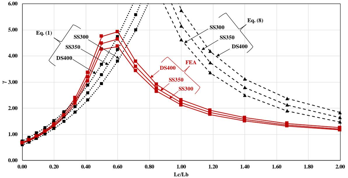
Figure 7: Buckling load predictions for the systems with  $L = 75\text{m}$
