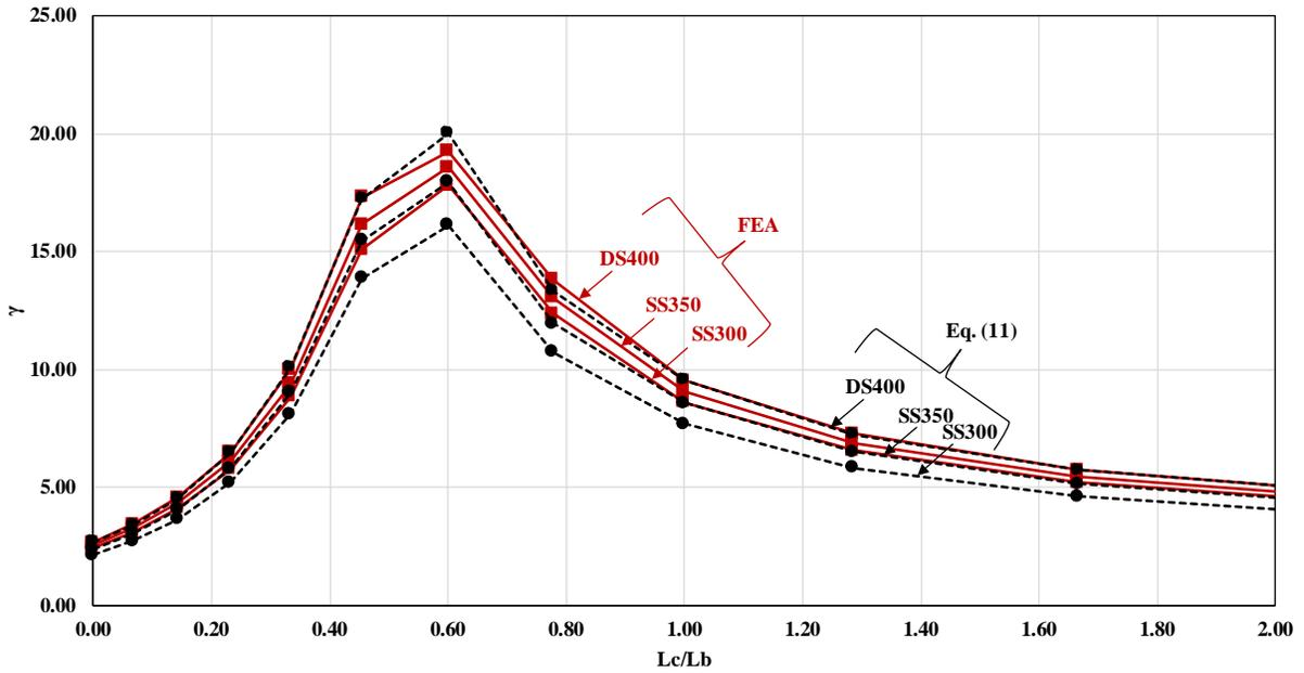
Figure 9: Buckling load predictions for the systems with  $L = 50\text{m}$  obtained with the proposed method
