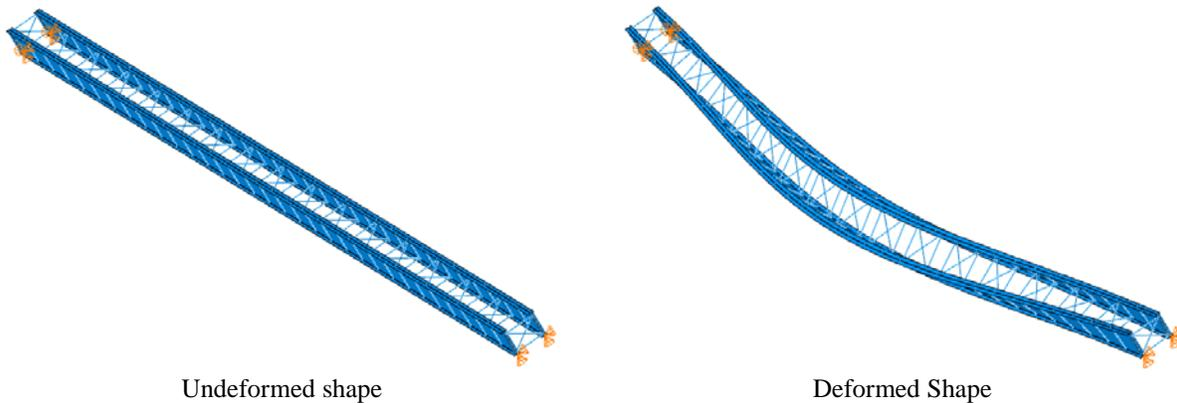
Figure 1: Global lateral – torsional buckling of a twin-girder system subject to a uniformly distributed load
