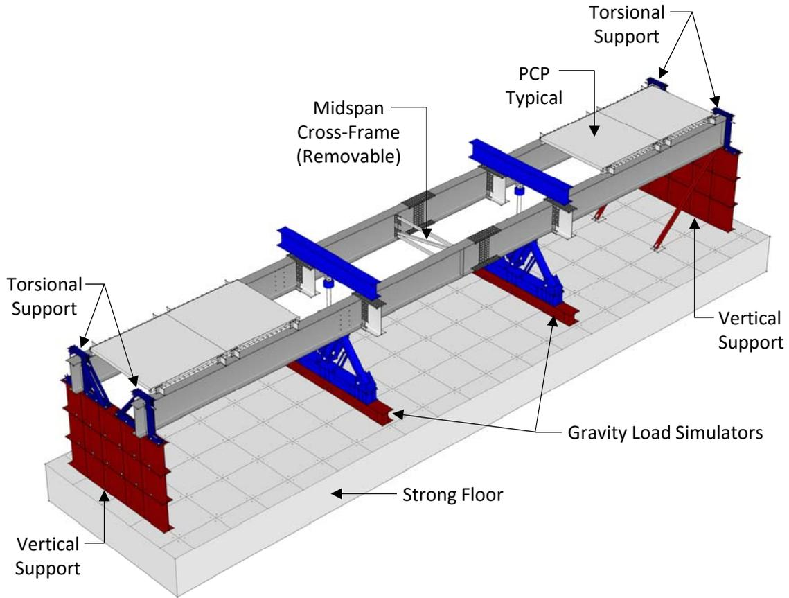
Figure 12: Twin I-Girder Combined Bending and Torsion Test Set-Up
