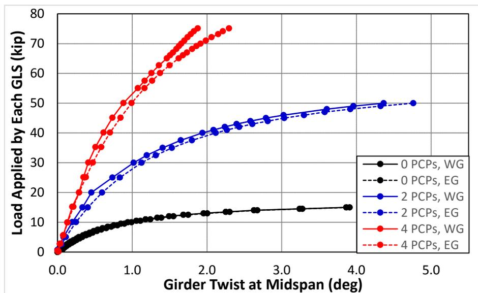
Figure 14: Midspan Girder Twist with Concentric Load, No Intermediate Cross-Frame and Varying PCPs
