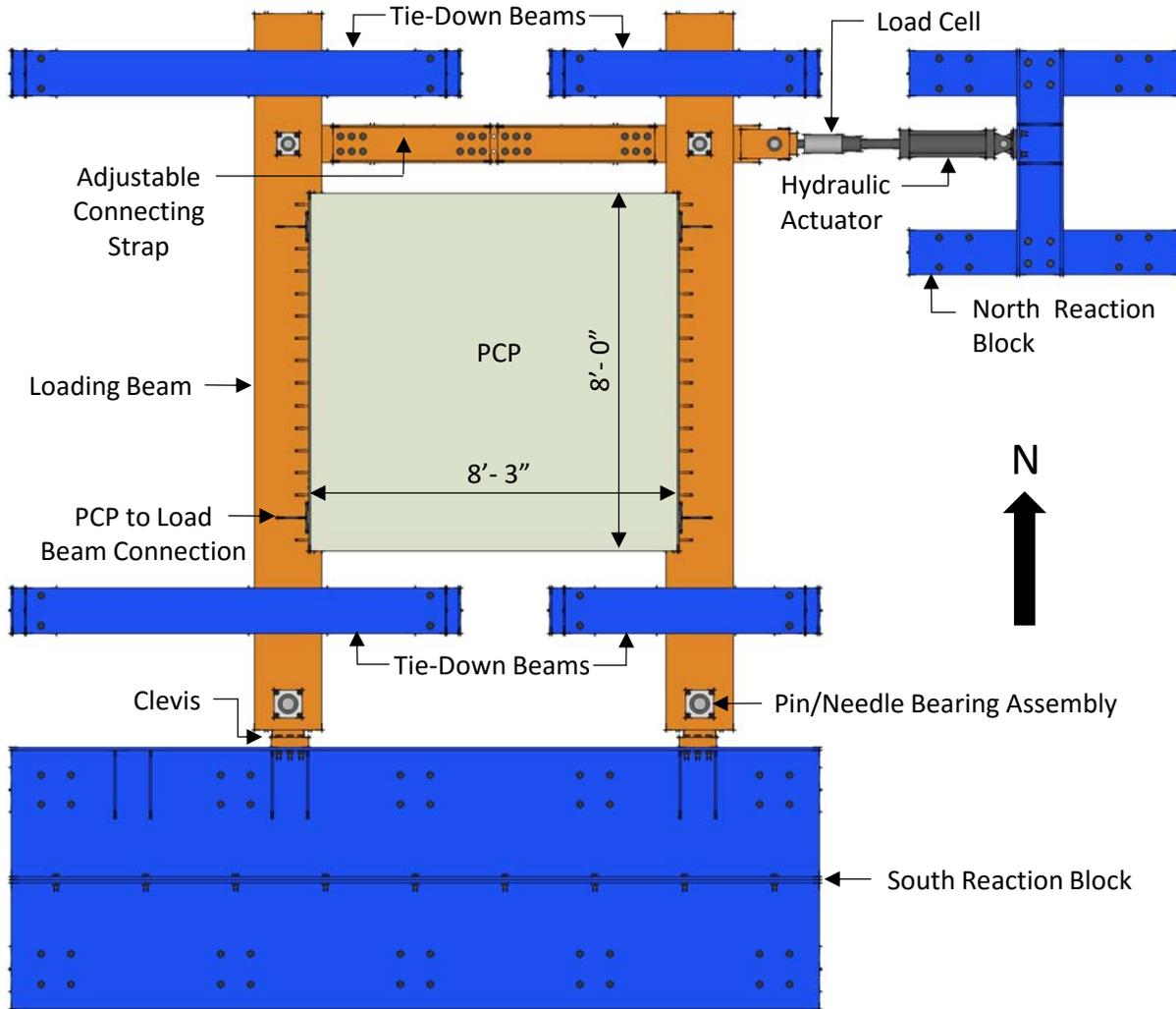
Figure 3: Shear Test Frame Plan View
