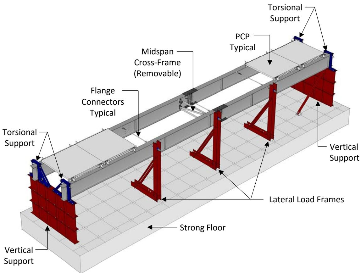
Figure 8: Twin I-Girder Lateral Test Set-Up
