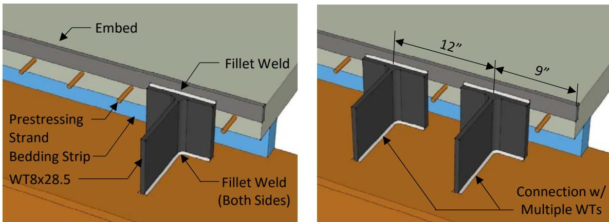
Figure 4: Detail of PCP Connection to Top Flange
