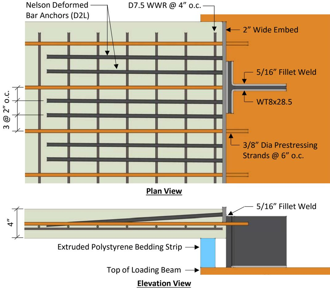
Figure 5: Plan and Elevation Views of the Embed-Anchor Detail
