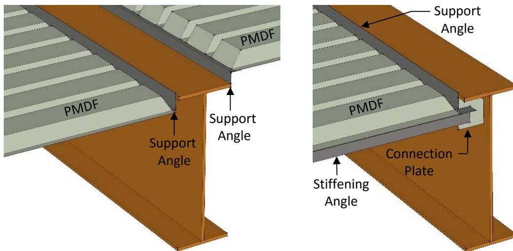
Figure 2: (a) Unstiffened PMDF Connection – Left (b) Stiffened PMDF Connection – Right
