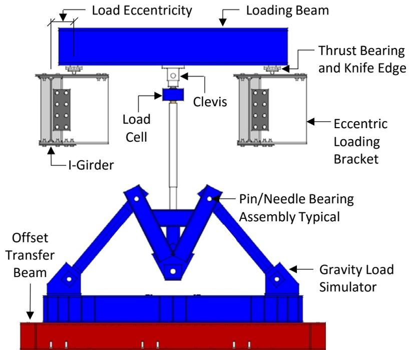
Figure 13: Twin I-Girder Vertical Loading System
