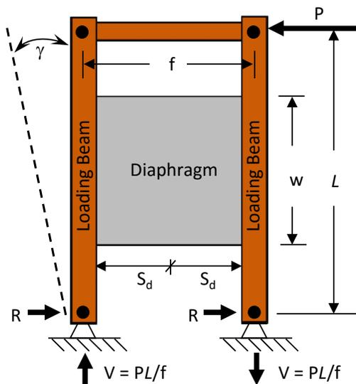
Figure 1: Shear Test Frame with Diaphragm
