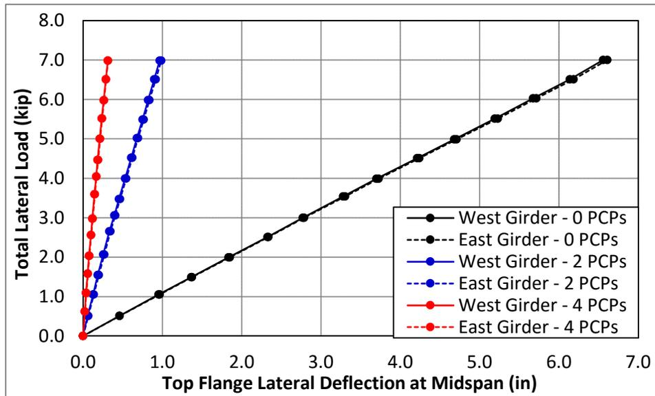
Figure 9: Midspan Deflection of Girders with Various Numbers of Attached PCPs
