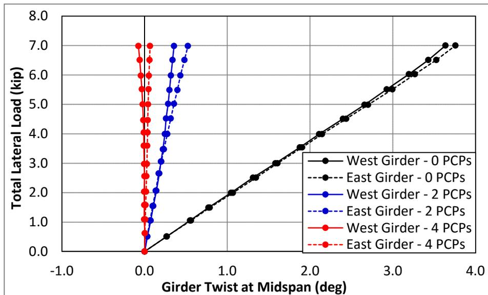
Figure 10: Midspan Twist of Girders with Various Numbers of Attached PCPs
