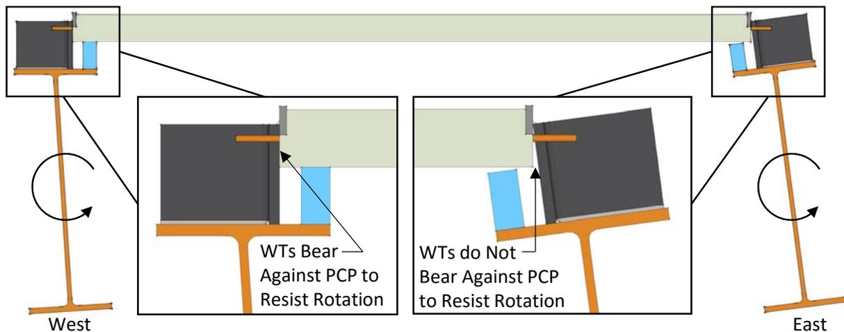
Figure 16: PCP to Top Flange Connection for the West and East Girders
