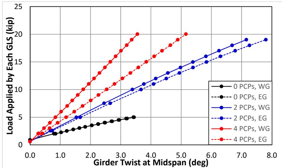
Figure 15: Midspan Girder Twist with 12" Eccentric Load, No Intermediate Cross-Frame, and Varying PCPs
