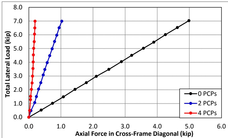
Figure 11: Forces in Cross-Frame Diagonal with Various Numbers of Attached PCPs
