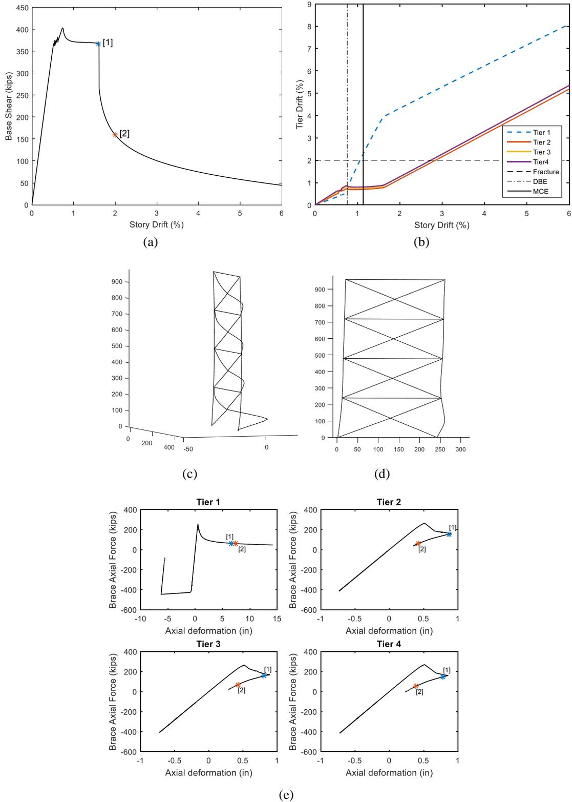
**Figure 4.** Response of OCBF10-4X-U (a) Base shear vs. story drift (pushover curve); (b) Tier drift vs. story drift; (c) Profile view of displaced shape at point [1]; (d) Elevation view of displaced shape at point [2]; (e) Brace response (positive indicates compression and axial shortening).
