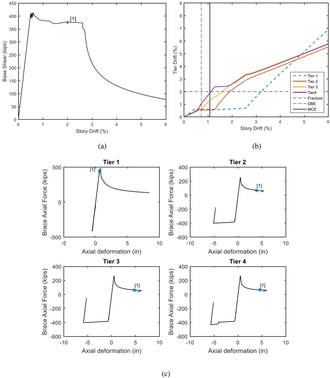
**Figure 8.** Response of OCBF10-4X-NU (a) Base shear vs. story drift (pushover curve); (b) Tier drift vs. story drift; (c) Brace response (positive indicates compression and axial shortening).
