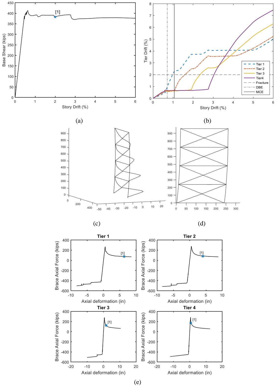
**Figure 5.** Response of OCBF16-4X-U (a) Base shear vs. story drift (pushover curve); (b) Tier drift vs. story drift; (c) Profile view of displaced shape at point [1]; (d) Elevation view of displaced shape at point [1]; (e) Brace response (positive indicates compression and axial shortening).
