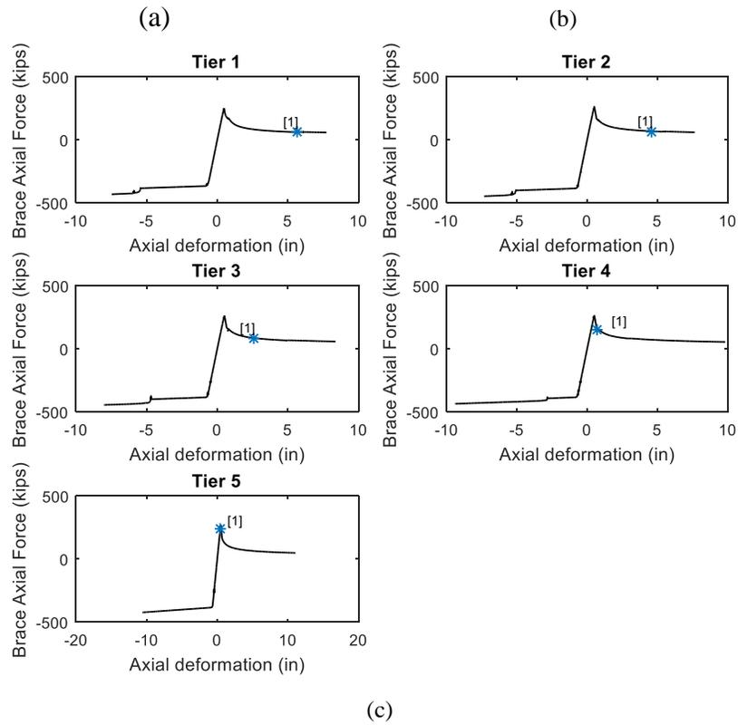
**Figure 7.** Response of OCBF16-5X-U (a) Base shear vs. story drift (pushover curve); (b) Tier drift vs. story drift; (c) Brace response (positive indicates compression and axial shortening).
