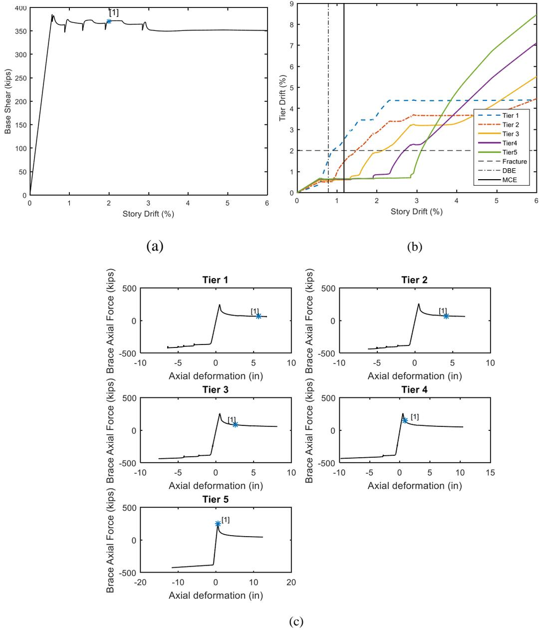
**Figure 6.** Response of OCBF10-5X-U (a) Base shear vs. story drift (pushover curve); (b) Tier drift vs. story drift; (c) Brace response (positive indicates compression and axial shortening).
