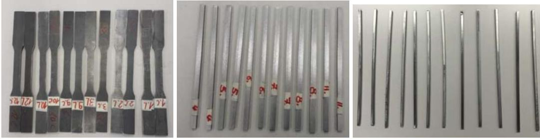
Figure 3: Tensile coupons extracted from – a) flat faces of cold-formed RHS sections – b) corners of cold-formed RHS sections – c) corners of hot-rolled CHS
