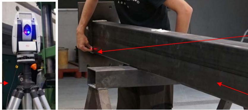
Reflector moving along the column length
