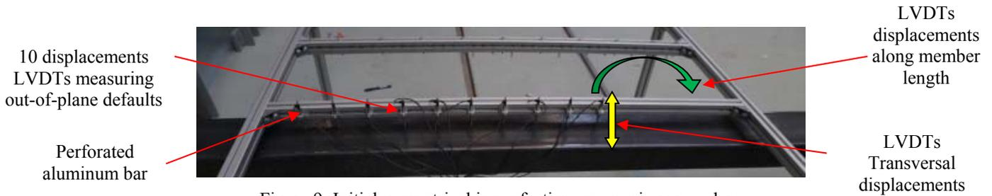
Figure 9: Initial geometrical imperfections measuring procedure
