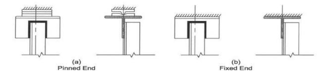
Figure 4: Test End Conditions for Single-Angle Struts
