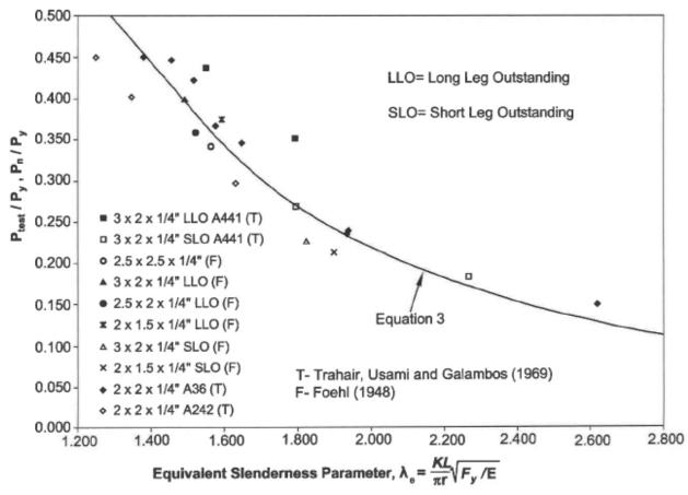
Figure 6: Equation 15 Shown as Equation 3 as Compared to Pinned-end Test Results
