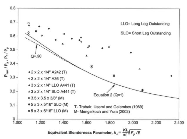
Figure 5: Equation 14 Shown as Equation 2 as Compared to Fixed-end Test Results
