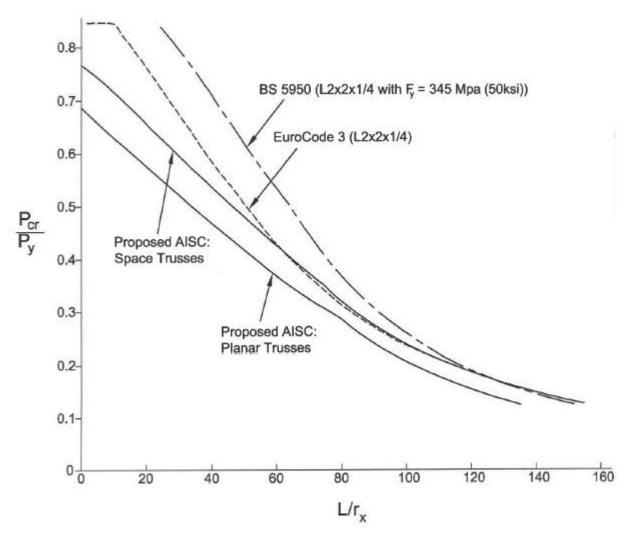
Figure 7: Comparison of Equivalent Slenderness Procedures for L2x2x1/4
