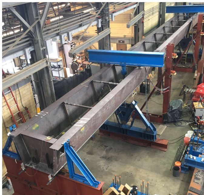
Figure 9 – Baseline Steel Tub Girder (No top lateral truss present) - Test Setup
