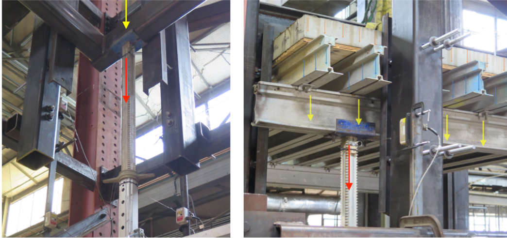
Figure 8: Load Application, Test No. 1 Left, Test No. 2, Right
