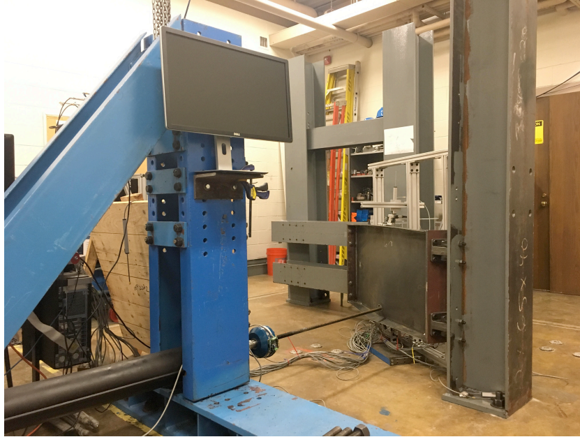
Figure 3: Metal building primary frame test setup with rod anchor
