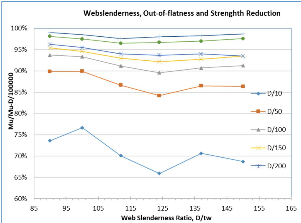
Figure 17: Normalized Ultimate Strength ( $M_u/M_{u,D/100,000}$ ) vs. Web Slenderness ( $\frac{D}{t}$ ) for Unstiffened I-Shaped Steel Plate Girders.
