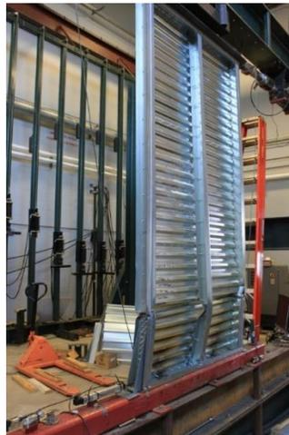
Fig. 7: Failures of the Shear Wall Specimen in Cyclic Test
