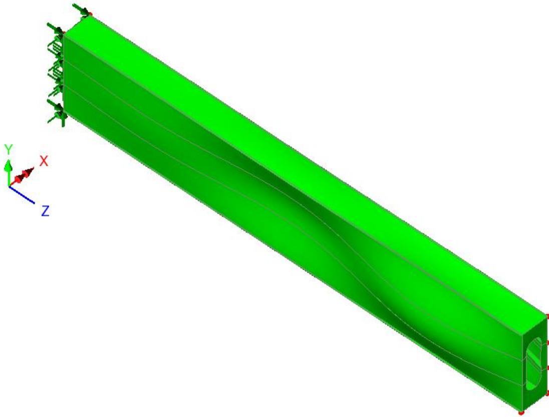
Figure 3: Deflected Arch Rib Model for Local Buckling Analysis
