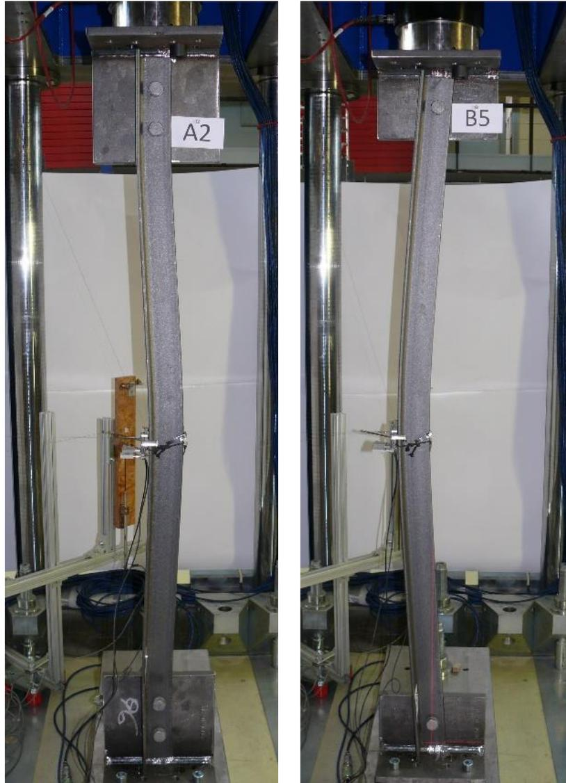
Figure 9: Member buckling tests for specimen A2 (two-bolt connection) and specimen B5 (one-bolt connection)
